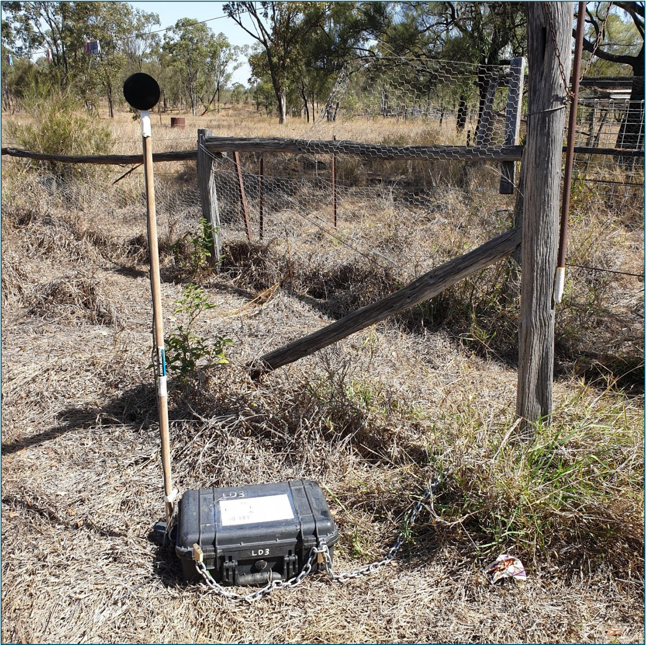
Figure B.1 Noise Logger setup at Receptor 6
