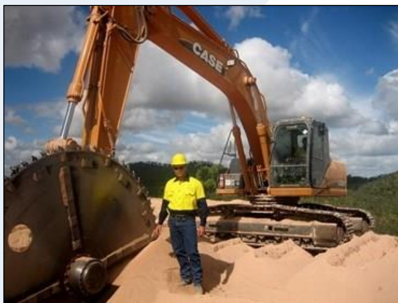
Figure 2. Excavator mounted stone saw.
