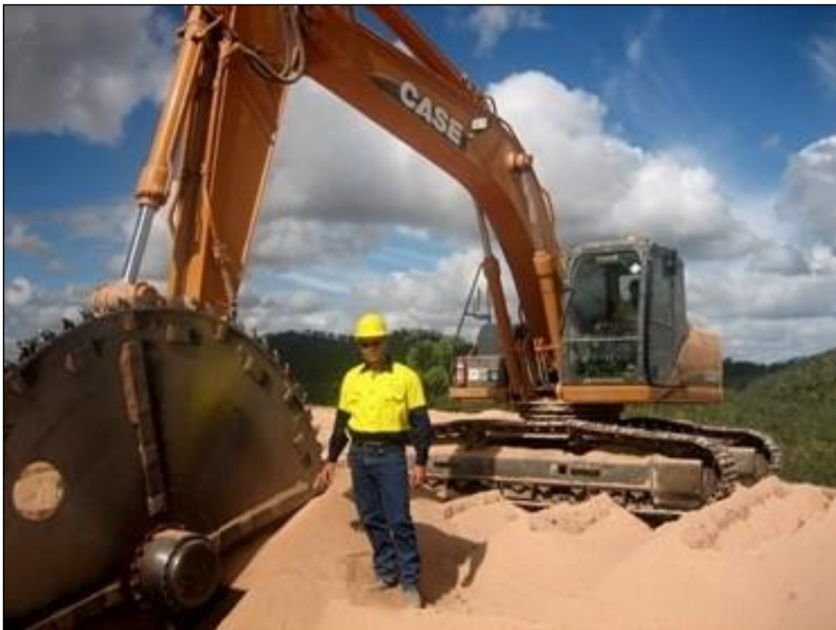
Figure 10. Excavator mounted saw.
