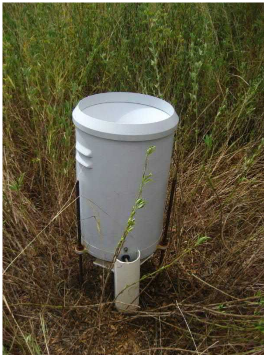
Automatic weather station – tipping bucket rain gauge
