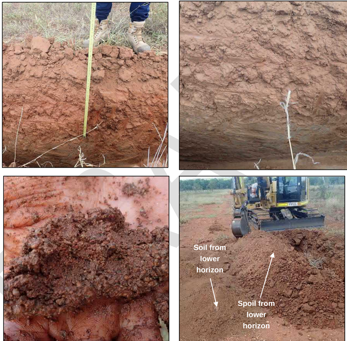
Figure 3: Photos Showing the Typical Condition of the Remainder of the Test Pits
