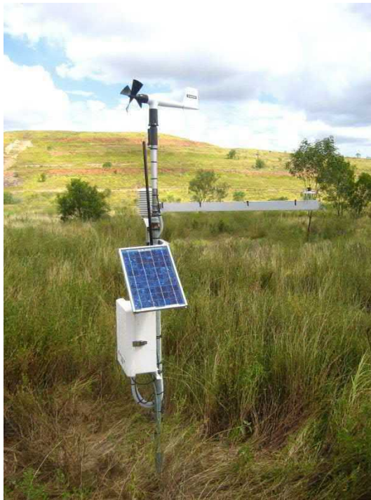
Automatic weather station
