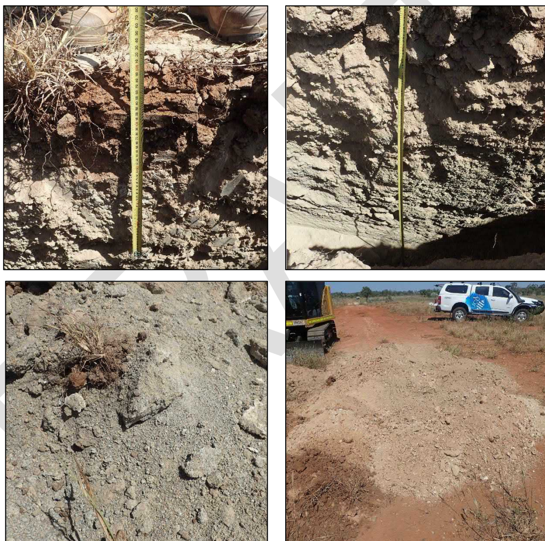
Figure 2: Photos Showing the Typical Condition of Test Pits 4 and 5
