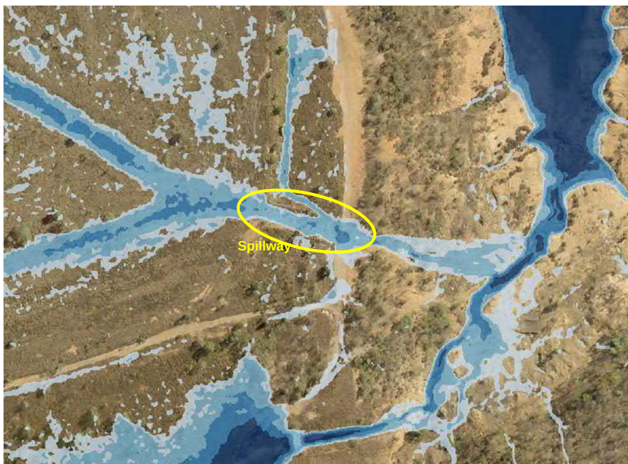
Figure 1.64: 1:1,000 AEP Peak Flood Extent for Spillway at Eastern Side of NNTSF
