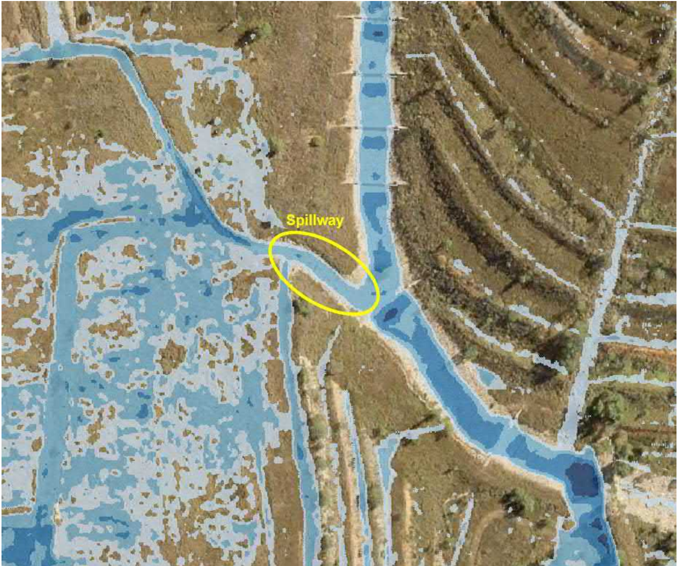
Figure 1.67: 1:1,000 AEP Peak Flood Extent for Spillway at North-Eastern Corner of STSF
