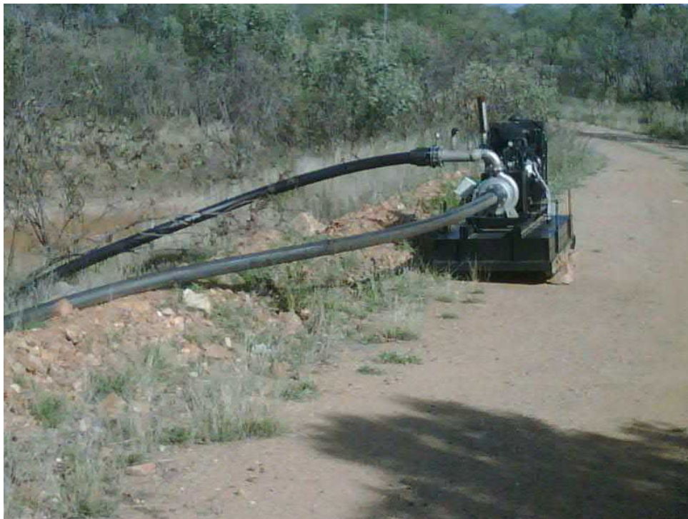
Western Scats Sump diesel pump
