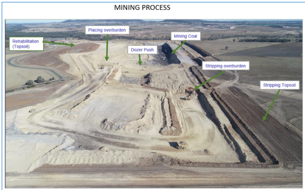
Figure 21 - Mining process from topsoil stripping to replacement.
