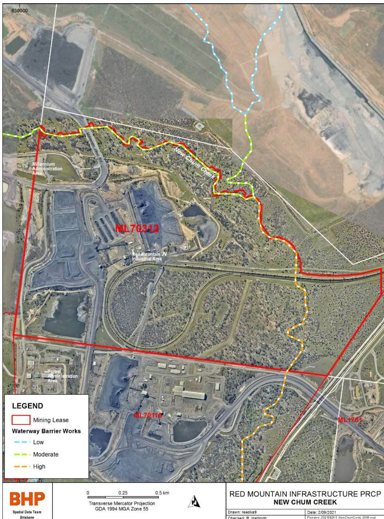
Figure 11: New Chum Creek watercourse (water barrier works delineation)
