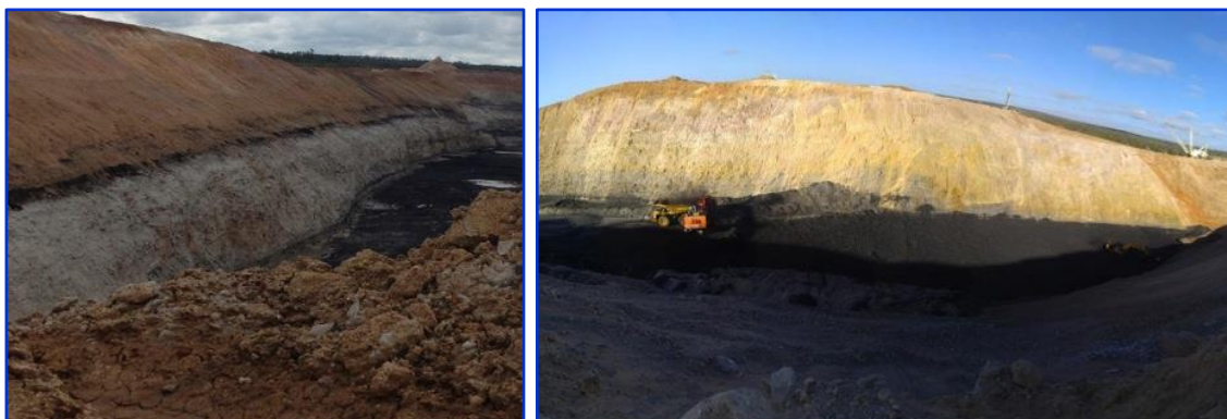
Figure 5-4 Tertiary spoil overlying Permian spoil in Y Pit (left) and F Pit (right)
