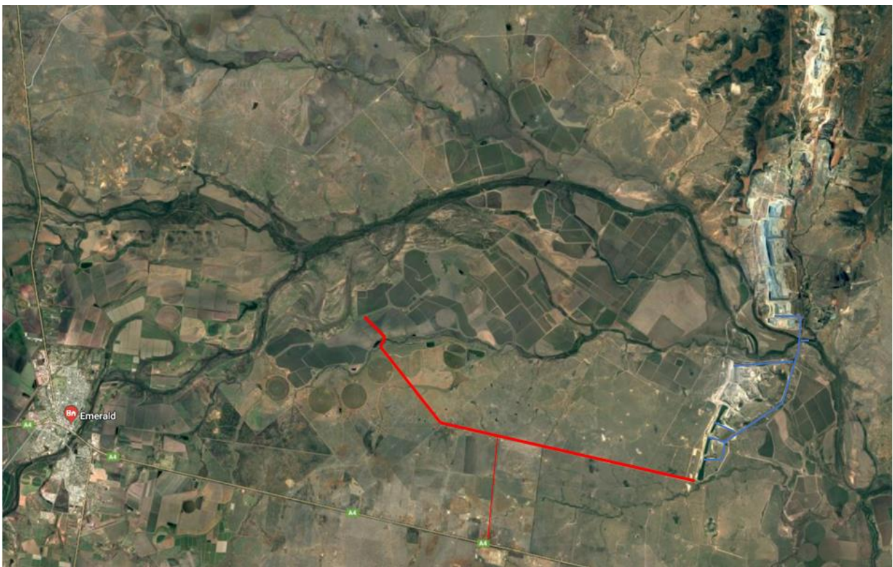
Figure 2.3 Conceptual drawing of the Weemah Channel and Yamala Inland Port pipeline connection (red) and the mine internal pump system (blue)
