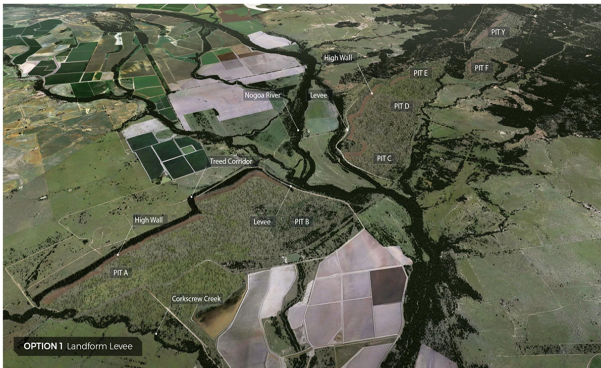
Figure 3-1: Option 1 - Landform levee
