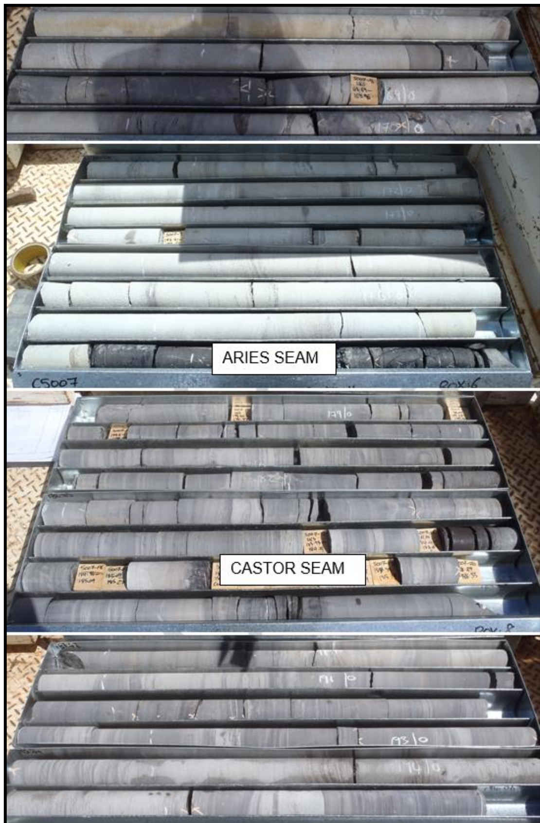
Figure 38. Castor Seam Stone Roof and Floor – Borehole C5007, 4002 Panel
