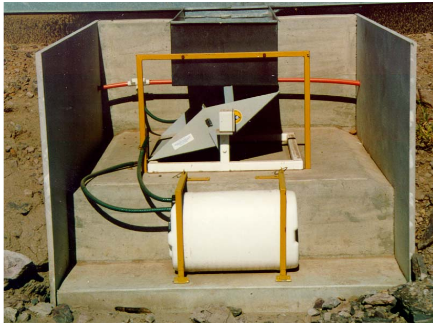
Figure 5-3 The tipping bucket and sampling apparatus for measurement of runoff, suspended load and water quality from a field plot at Oaky Creek mine.
