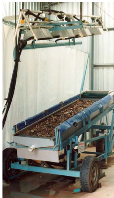
Figure 3-1 The erosion processes laboratory at The University of Queensland showing the tilting erosion flume and the rainfall simulator.
