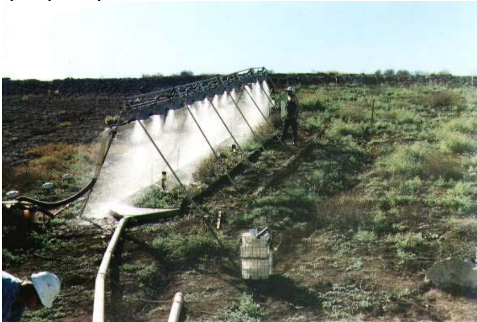
Figure 4-1: The rainfall simulator in use at the Curragh Mine
