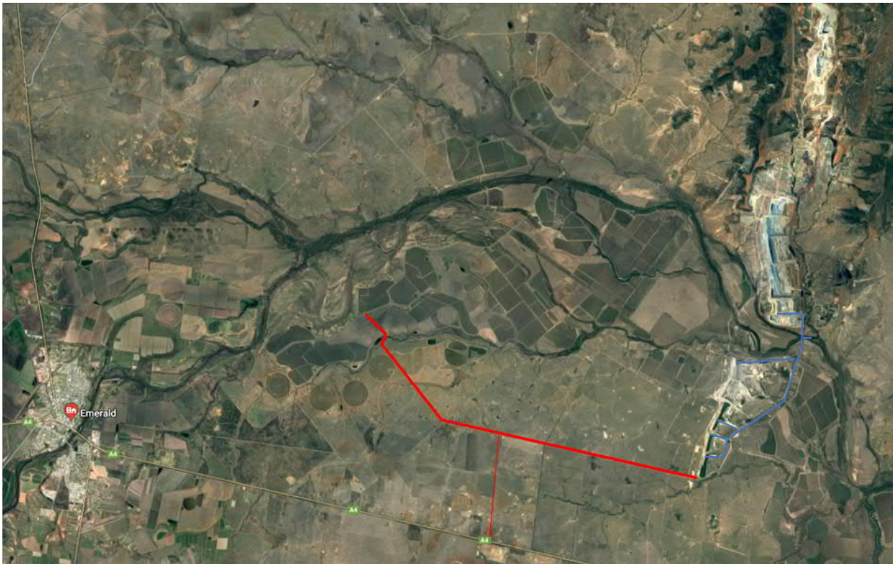
Figure 3. Conceptual drawing of the Weemah Channel and Yamala Inland Port (red) pipeline connection and the mine internal pump system (blue)
