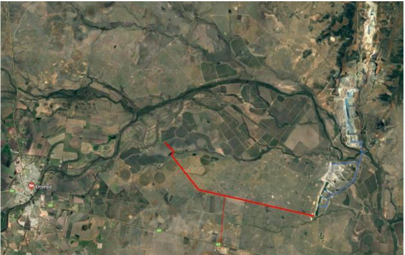
Figure 3 Conceptual Plan of the Weemah Virtual Channel to Irrigation and Yamala Inland Port (red) and the Mine Internal Pump System (blue)
