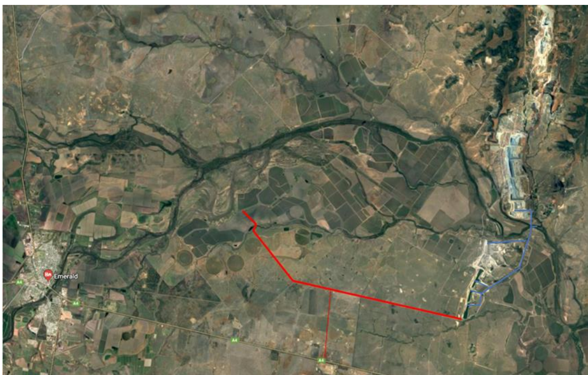
Figure 3.3 - Conceptual drawing of the Weemah Virtual Channel to irrigation and Yamala Inland Port (red) and the mine internal pump system (blue)
