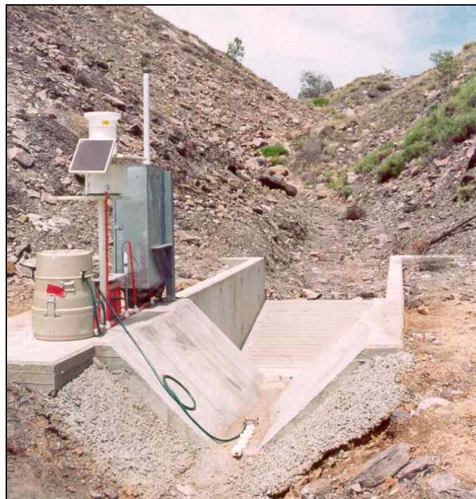
Figure 2. Catchment flume and sampling equipment.
