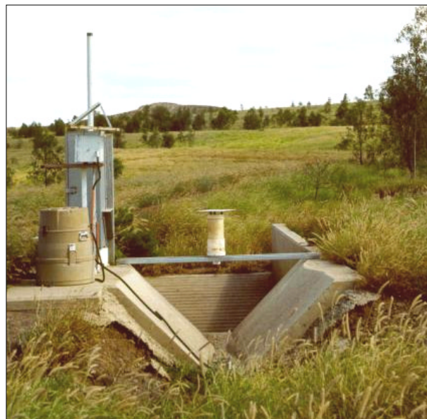
Figure 2. Catchment flume and sampling equipment.
