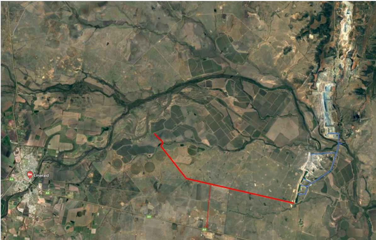
Figure 3.3 Conceptual drawing of the Weemah Channel and Yamala Inland Port (red) pipeline connection and the mine internal pump system (blue)
