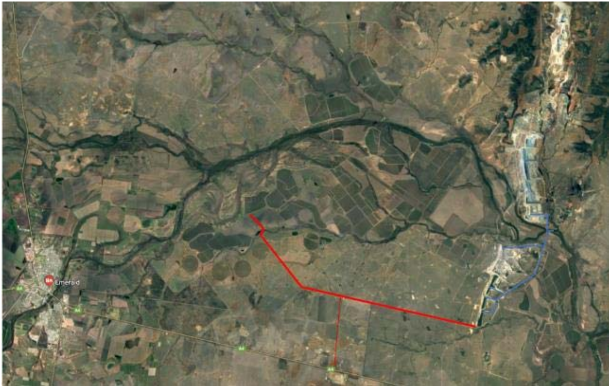
Figure 1-3: Conceptual drawing of the Weemah Virtual Channel to irrigation and Yamala Inland Port (red) and the mine internal pump system (blue)
