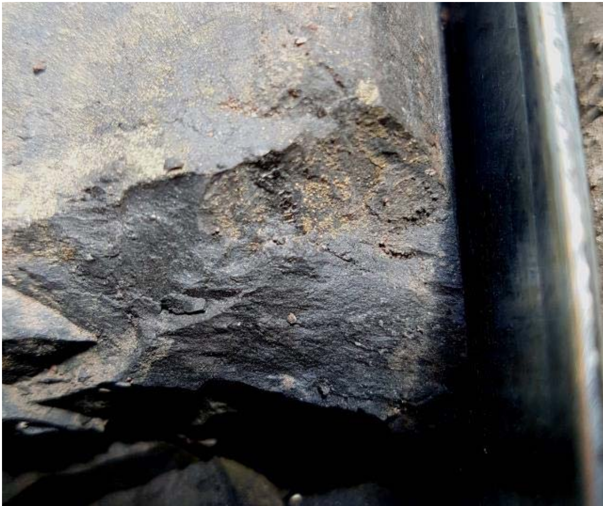
Figure 4-14: Pyrite in coal at approximately 65 m depth in drill hole C5286
