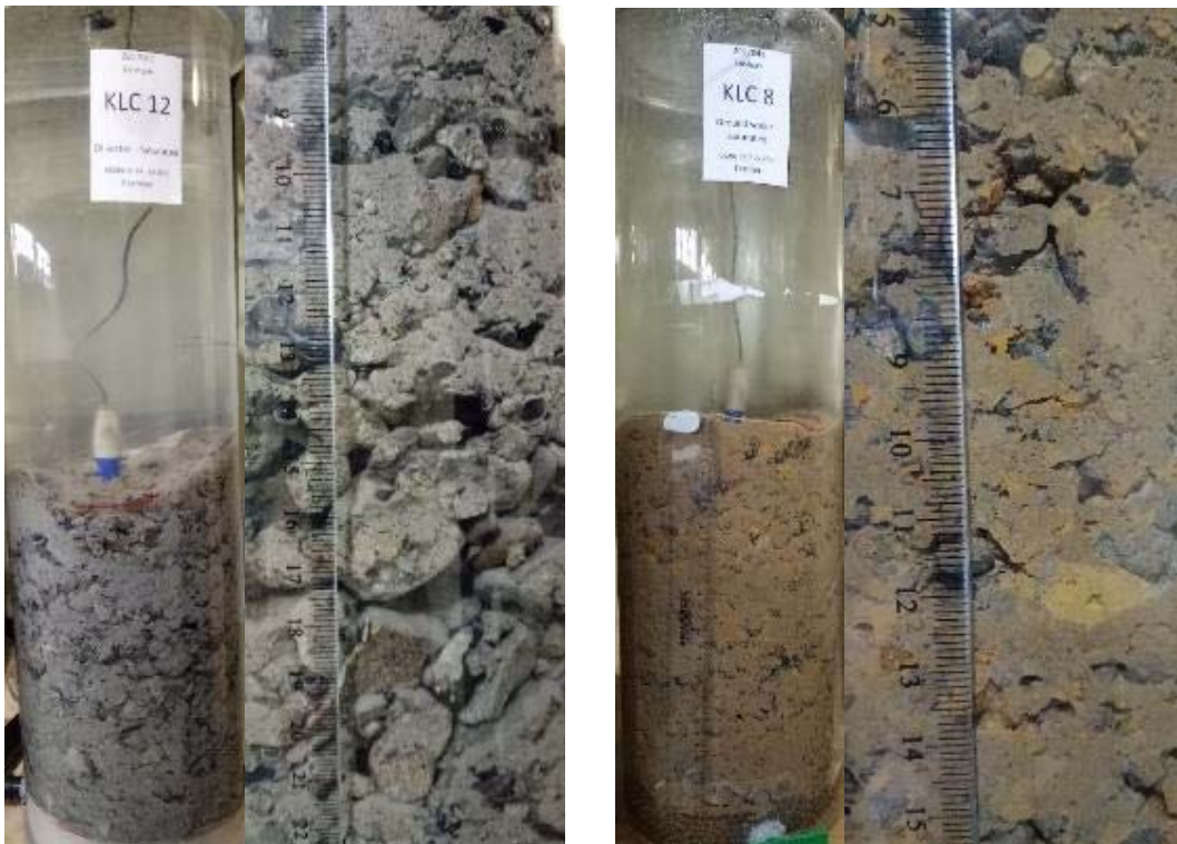
Figure 3-7: Y Pit Permian spoil (left) Quaternary/Tertiary Spoil (right)
