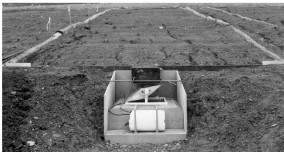
Fig. 2. Erosion plot and runoff tipping bucket; suspended sediment collected in 20-L plastic drum, via 1-mm slot in 10-cm upright copper pipe (left of tipping bucket).
