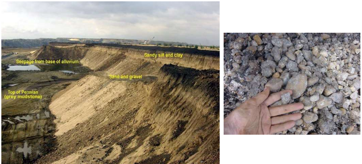
Figure 1 – LHS The typical alluvial profile as exposed in B Pit. RHS Gravel cuttings from base of bore EC14 – note fines have been washed from cuttings during drilling.
