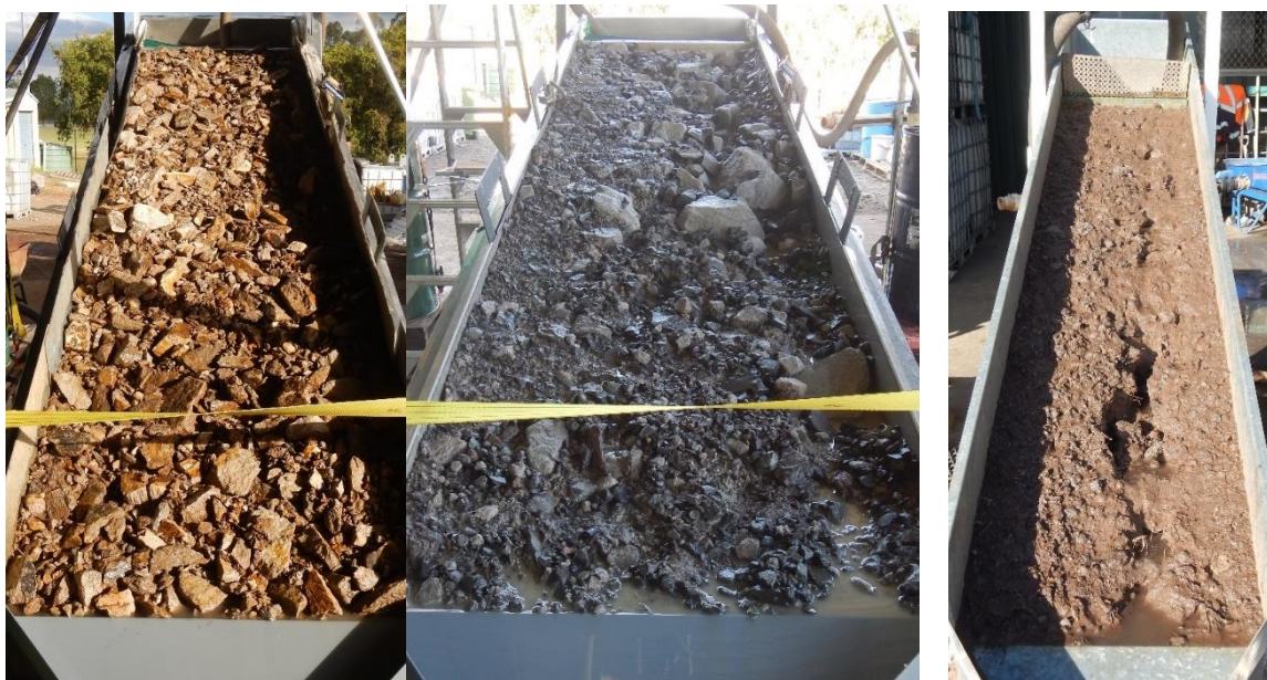
Figure 6: Flumes showing application of flow to (L-R) 4:1 Quarry rock:topsoil mix, 4:1 Permian rock:topsoil mix, and topsoil.
