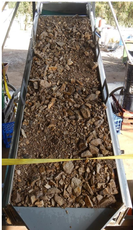
Figure 5: Surface of 4:1 Quarry rock:topsoil mix following application of simulated rain, 0.77 m wide flume.
