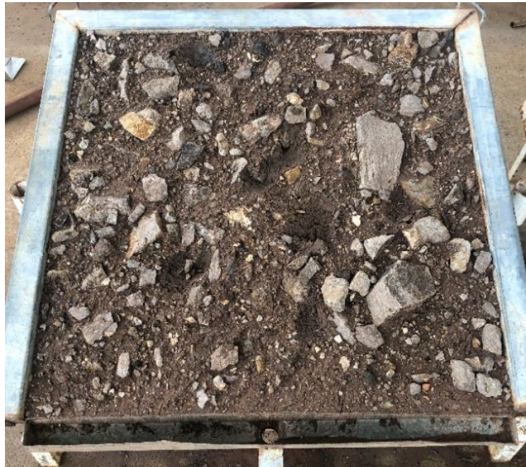
Figure 4: Surface of 2:1 Quarry rock:topsoil mix following application of simulated rain, 0.75 m wide plot.
