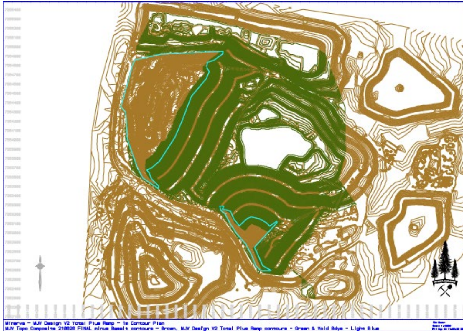
Figure 2 – Plan view of final void reshaping
