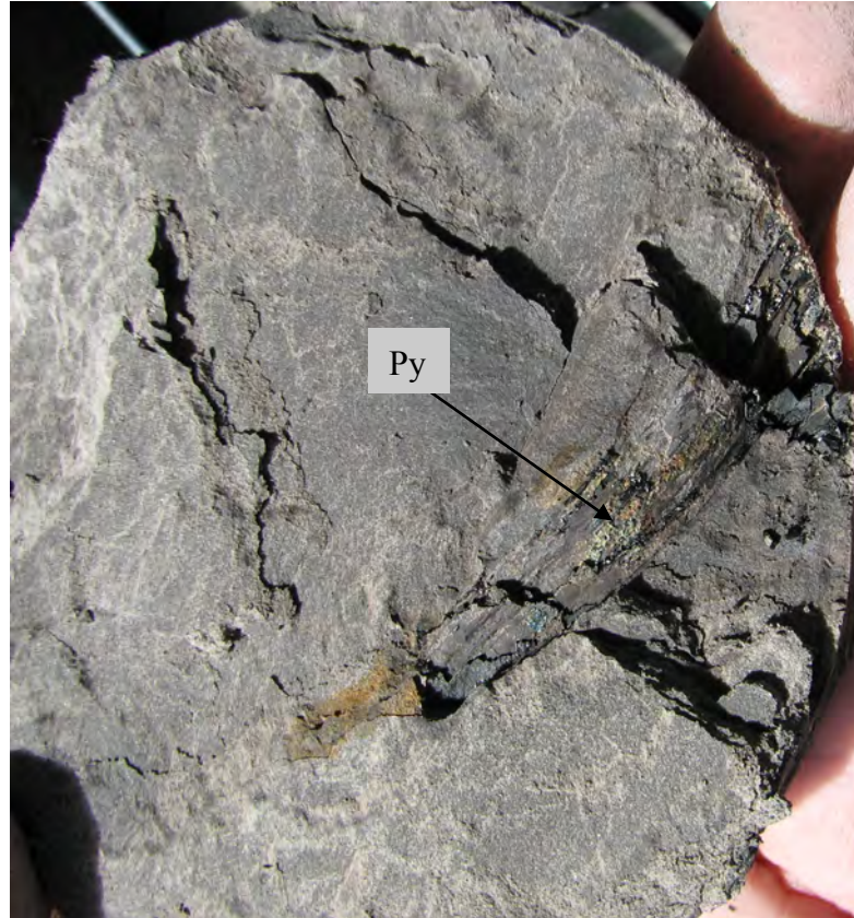
Plate 2: Minor pyrite coatings associated with leaf fossils. Hole C10_1 at 26.7m.
