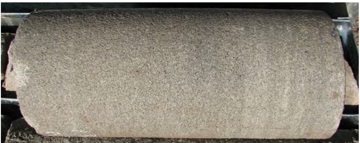
Plate 3: Sandstone with reactive carbonate in matrix. Hole C10_10 at 22.40m.
