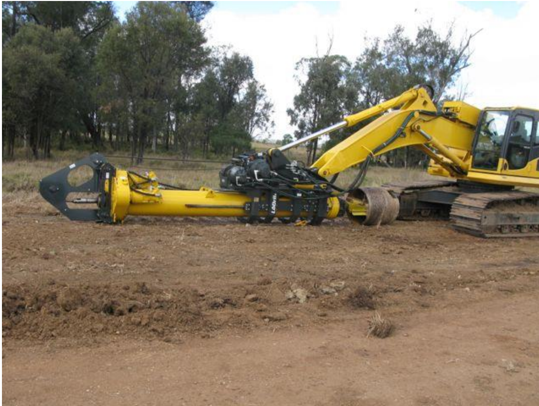
Figure 28: LoDrill used for Exploration
