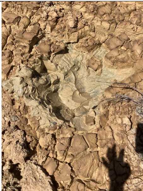
Figure 10: PL2 Wet Tails showing crusting
