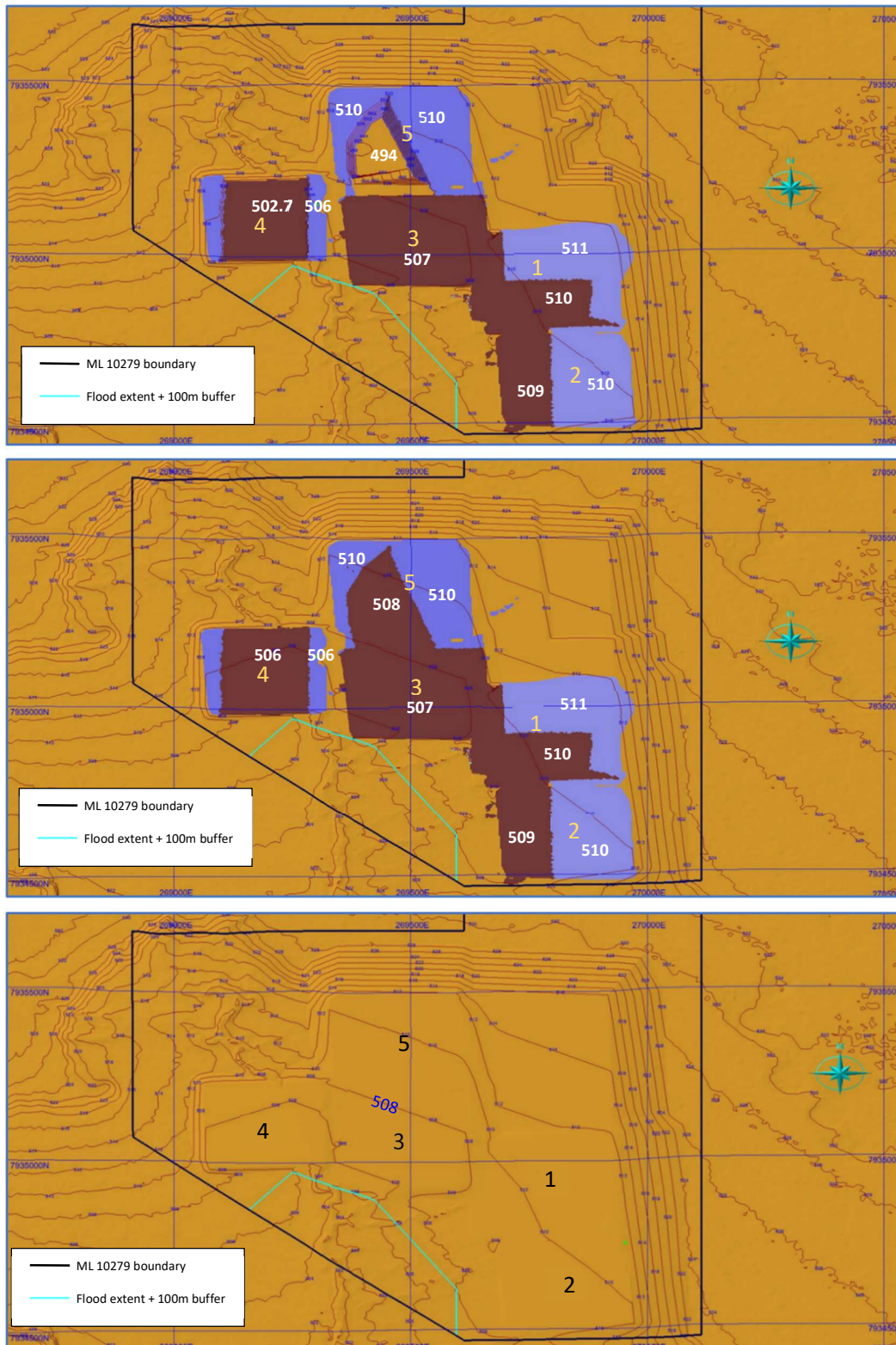
Figure 17 Pit 5 backfill and final landform profile
