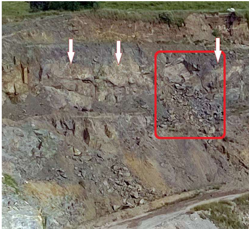
(a) Planar sliding of unweathered andesite along single discontinuities dipping out from the north wall.
