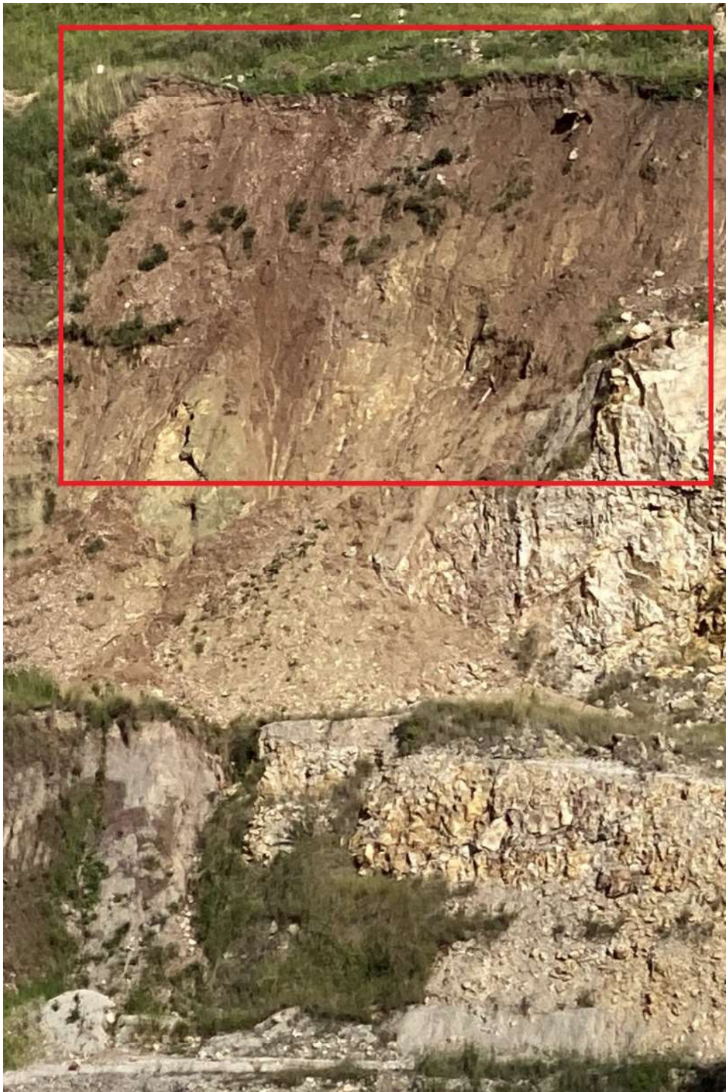
Figure 9. Typical bench scale rotational sliding failure through weathered andesite on the north wall.
