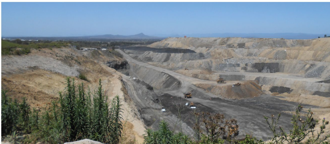
Figure 15: Oakleigh West: pre-rehabilitation—pit depth of approximately 90 m (2012)
