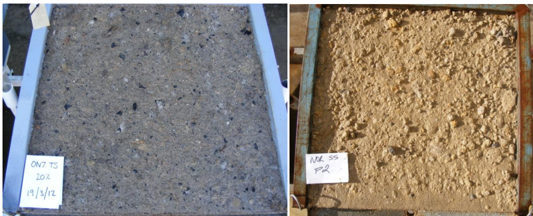
Figure 13: Rainfall simulator plots of ON7 topsoil (L) and NOR subsoil (R) following application of simulated rain.
