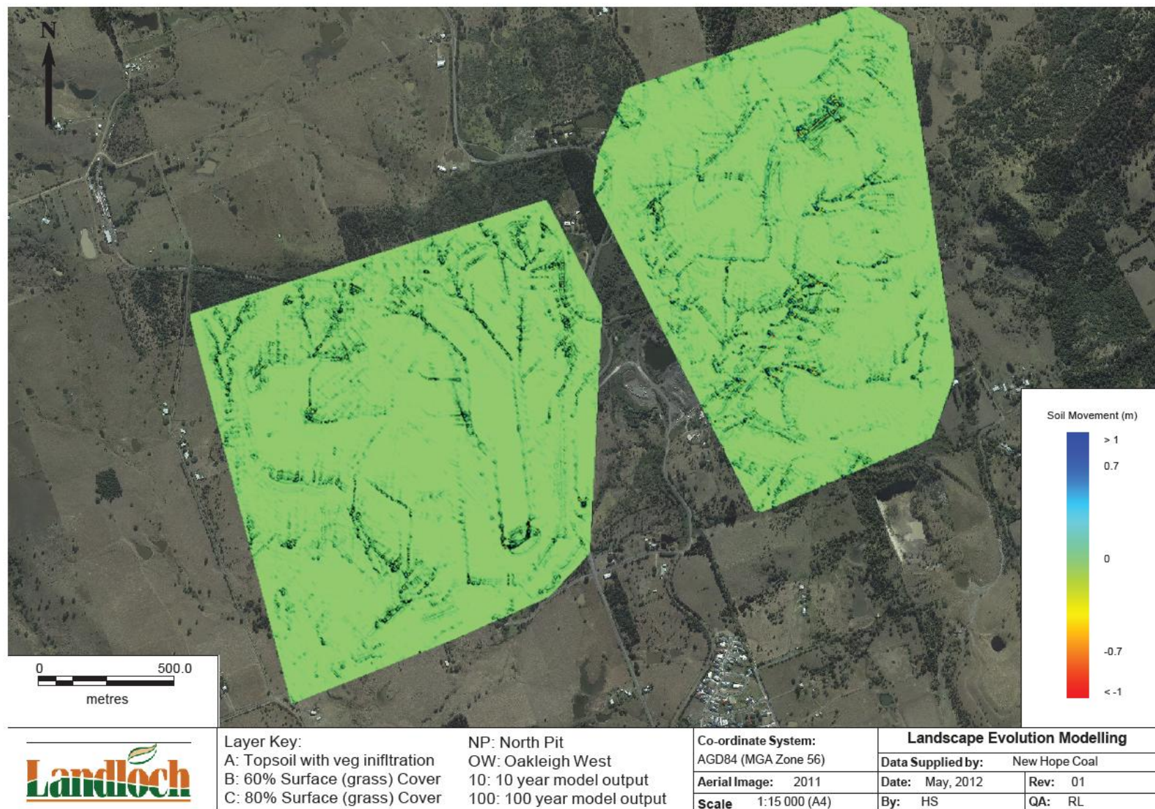
Figure 26: Predicted elevation change across Oakleigh West and North, 10-year simulation, 80% surface cover.
