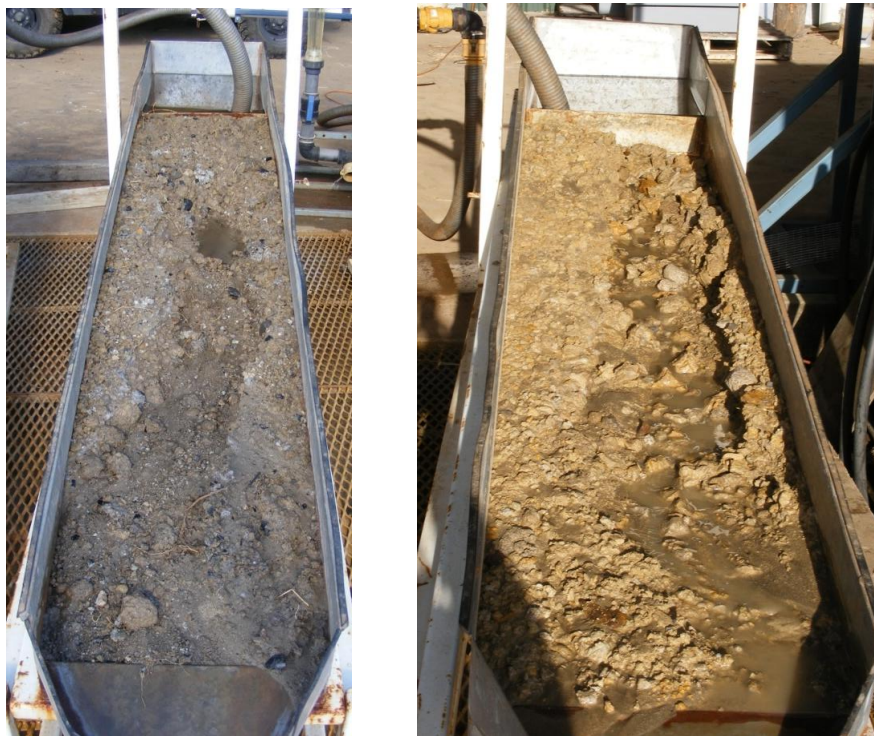
Figure 14: Flumes of ON7 topsoil (L) and NOR subsoil (R) following application of overland flows.
