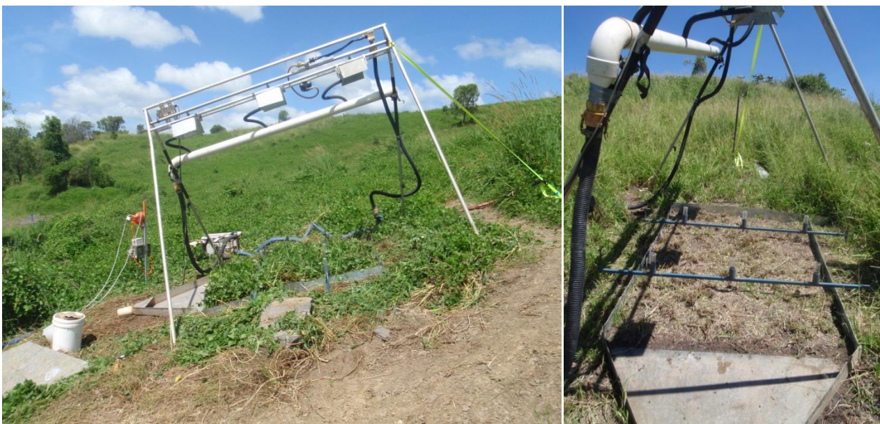
Figure 12: Rainfall simulator on Oakleigh North, showing vegetated plot (left) under heavy legume cover and clipped plot (right) in grassed area.
