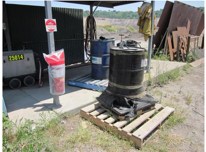
Photograph 14 – Fuel drums stored on wooden pallets, and storage of materials near to the wash down bay area (15/11/11).
