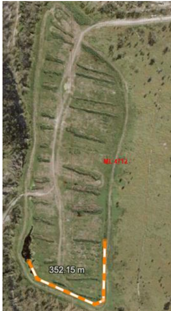
IMAGE 29: PROPOSED DRAIN ON COMPOSTING PAD
