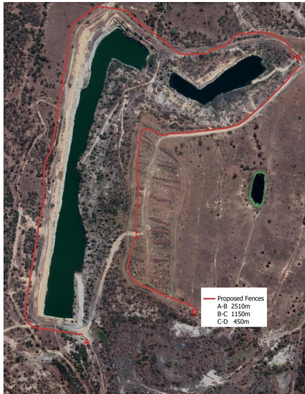
FIGURE 10: LOCATION OF STOCK FENCE AROUND VOIDS
