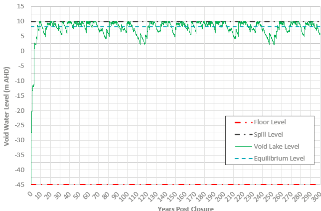
Figure 7.24 Final void water level time series results
