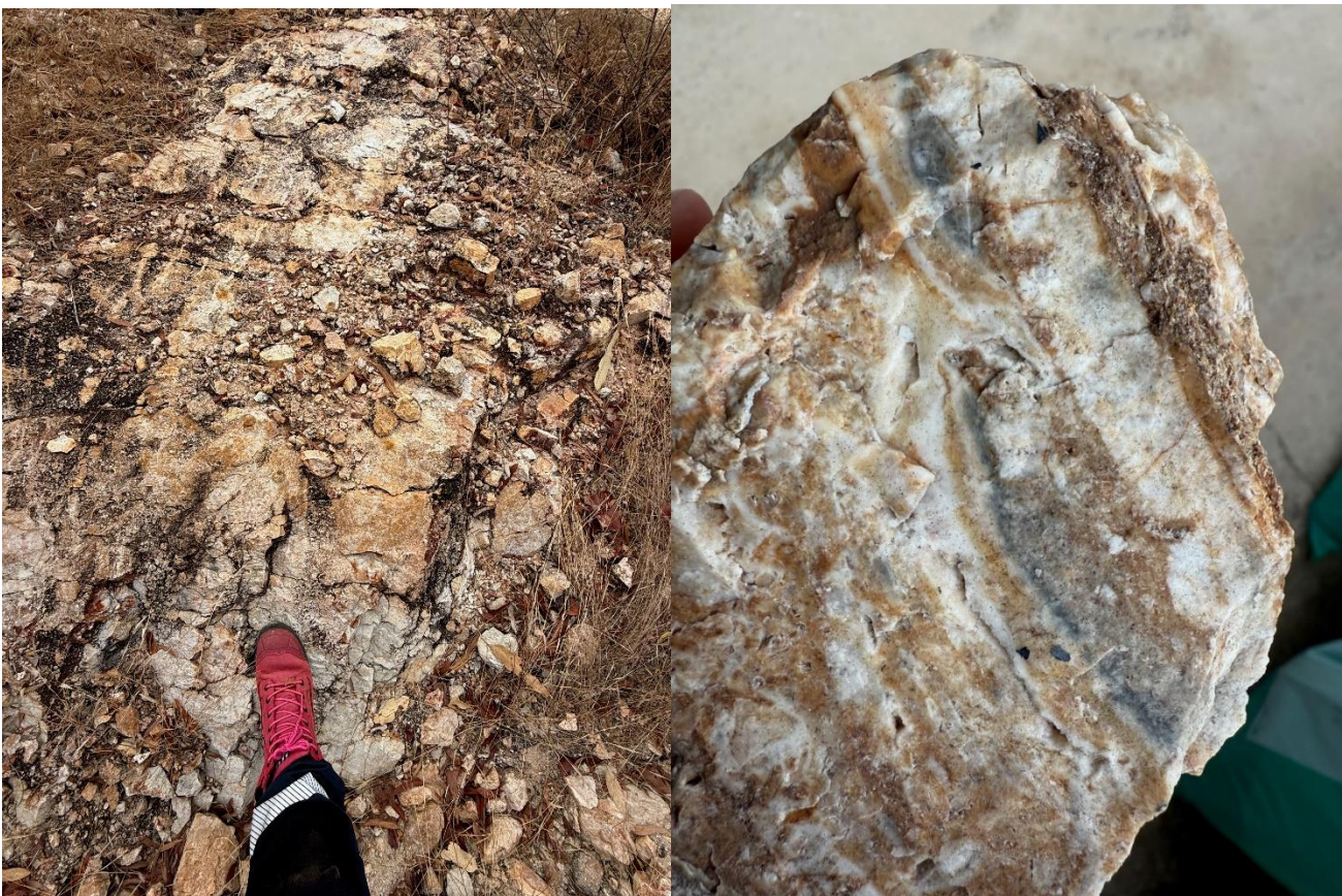
Figure 34 - View of weathered granite at surface, and example veining mineralisation with sulphides
