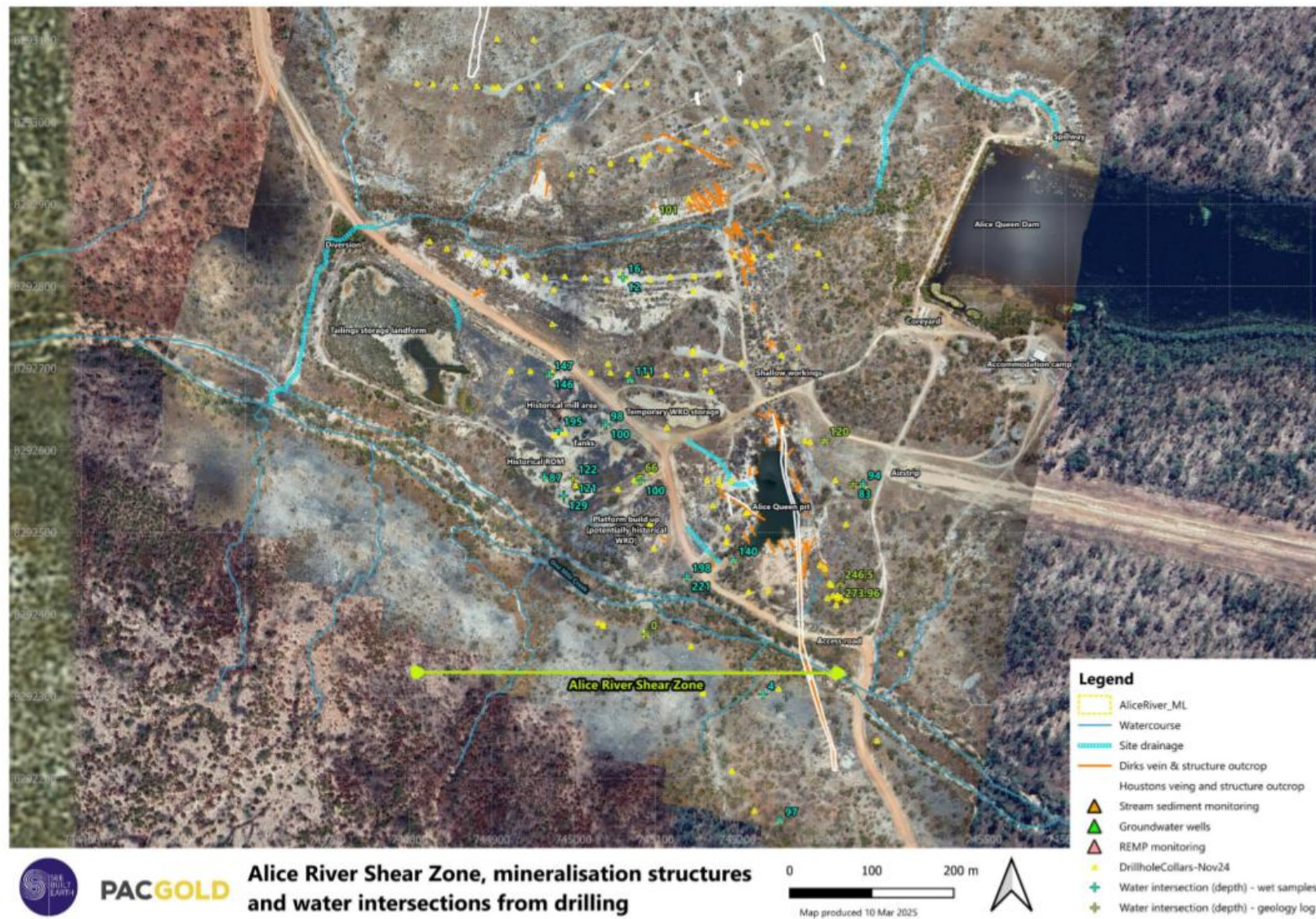
Figure 3-7: Alice River shear zone, mineralisation structures and water intersections from drilling
