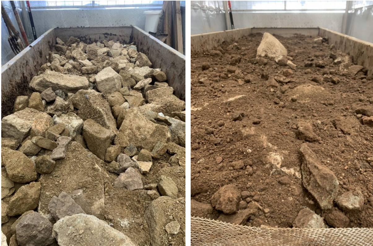
Figure 3-2: MRO RaE SIM Sample # 5 (West Hill saprock) + West Hill topsoil representing the proposed NWRD cover system
