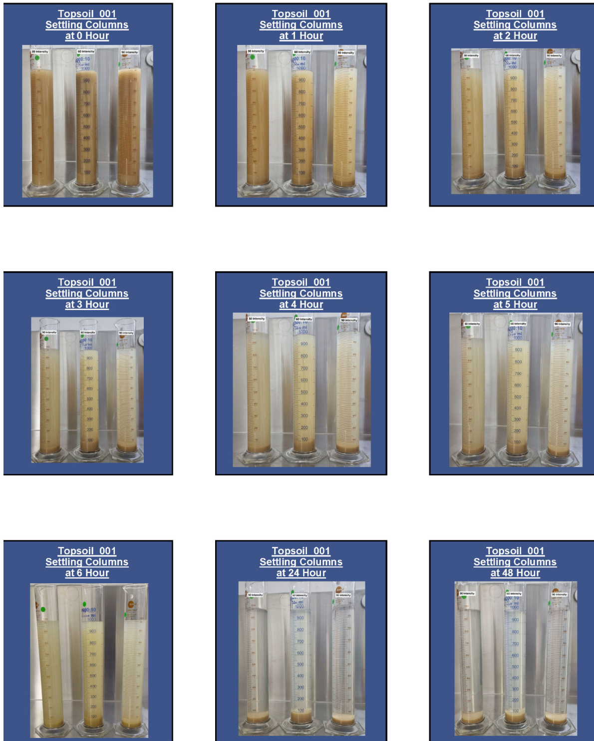
Figure 4-9: Suspended sediment settlement columns at 0 hours to 48 hours for MRO Sample #1.
