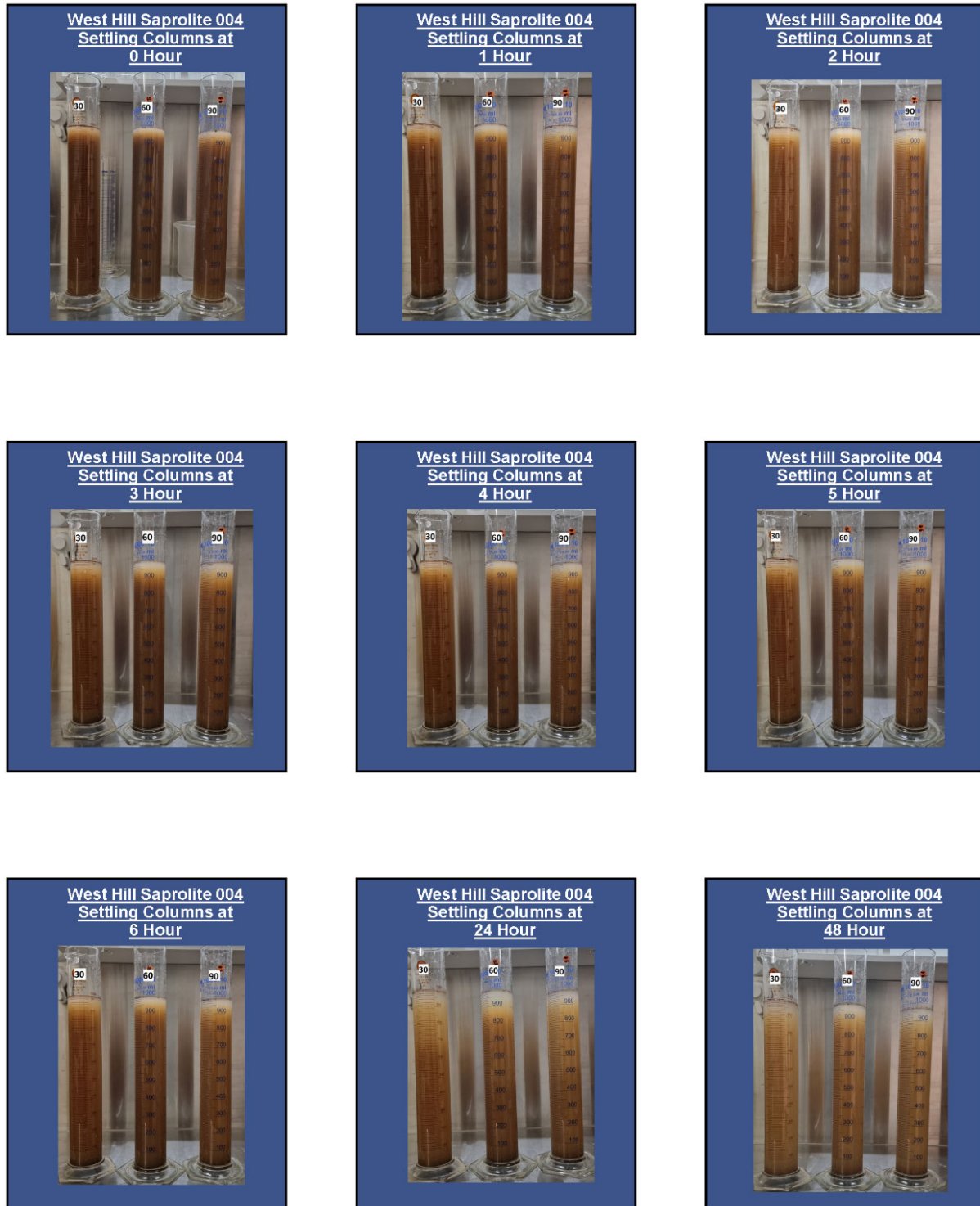
Figure 4-12: Suspended sediment settlement columns at 0 hours to 48 hours for MRO Sample #4.
