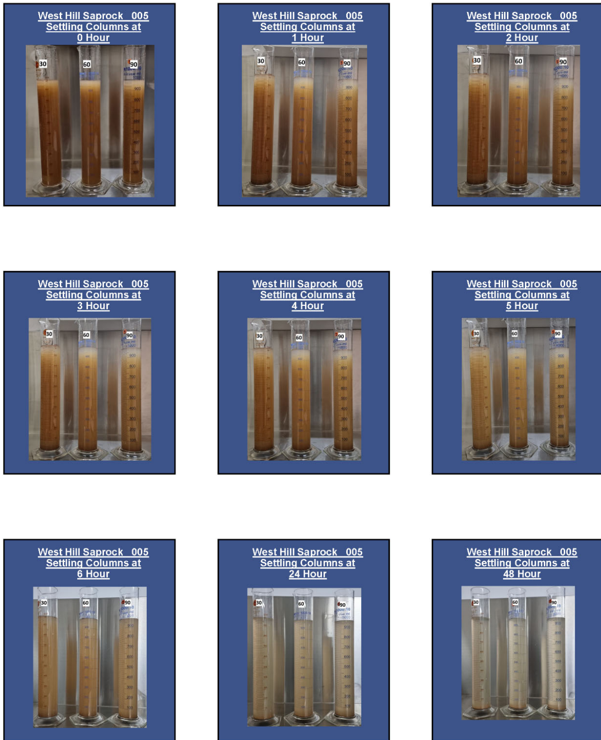
Figure 4-13: Suspended sediment settlement columns at 0 hours to 48 hours for MRO Sample #5.
