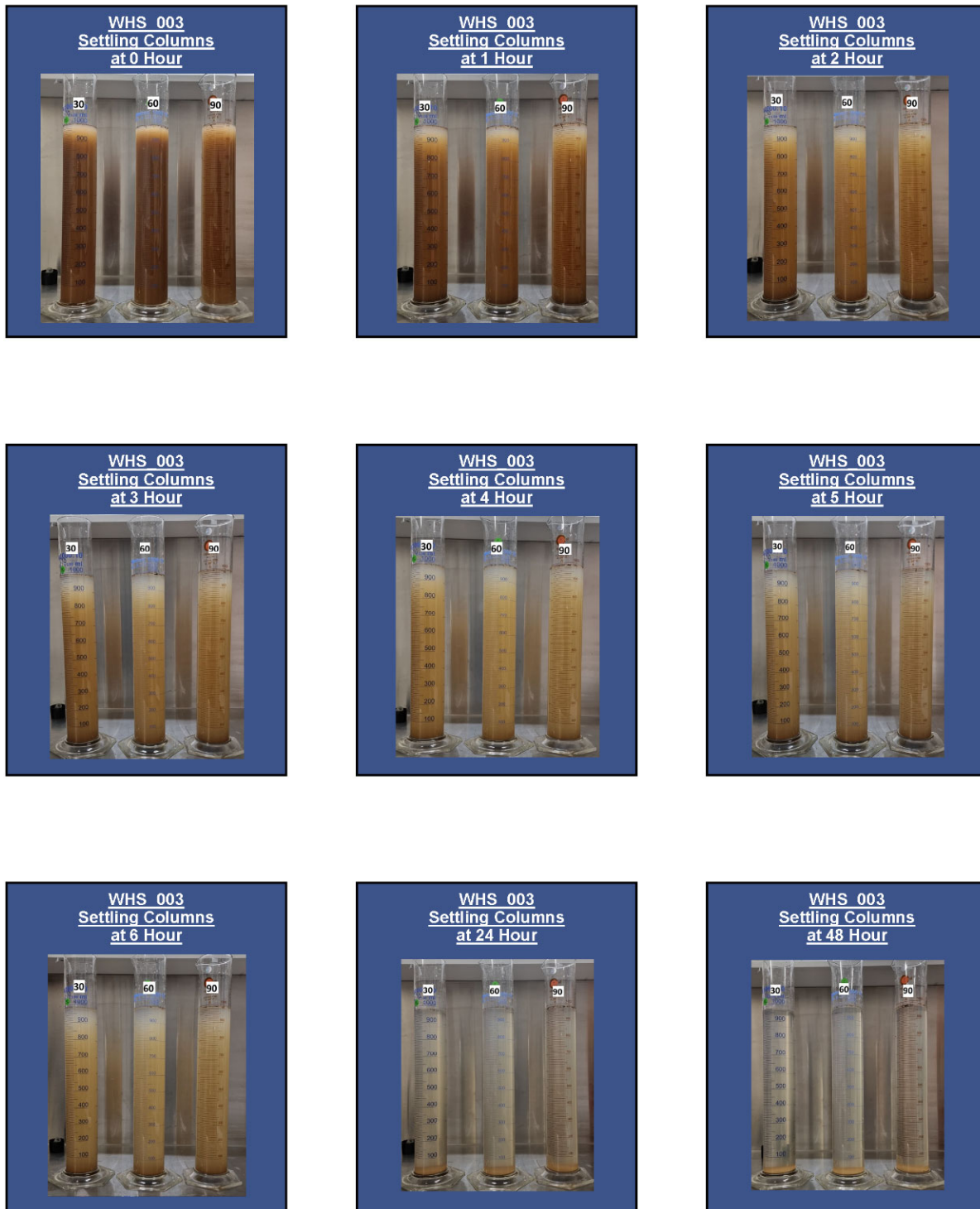
Figure 4-11: Suspended sediment settlement columns at 0 hours to 48 hours for MRO Sample #3.
