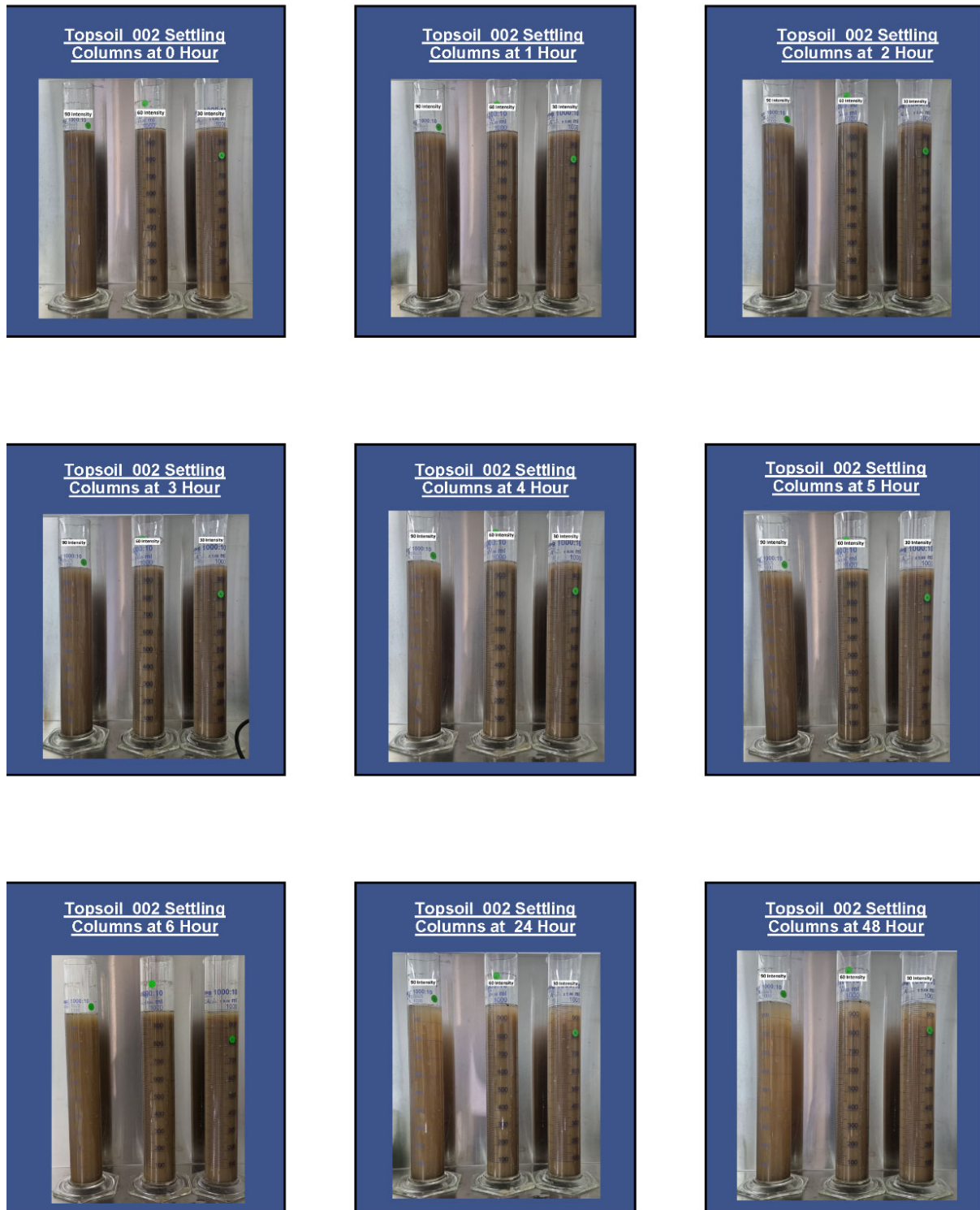
Figure 4-10: Suspended sediment settlement columns at 0 hours to 48 hours for MRO Sample #2.
