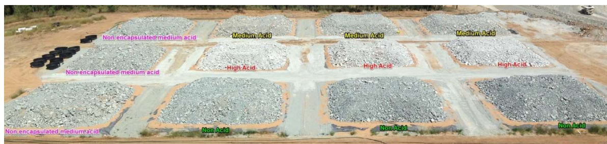
Figure 56 : Field waste rock lysimeter pads (ca. 2016).
