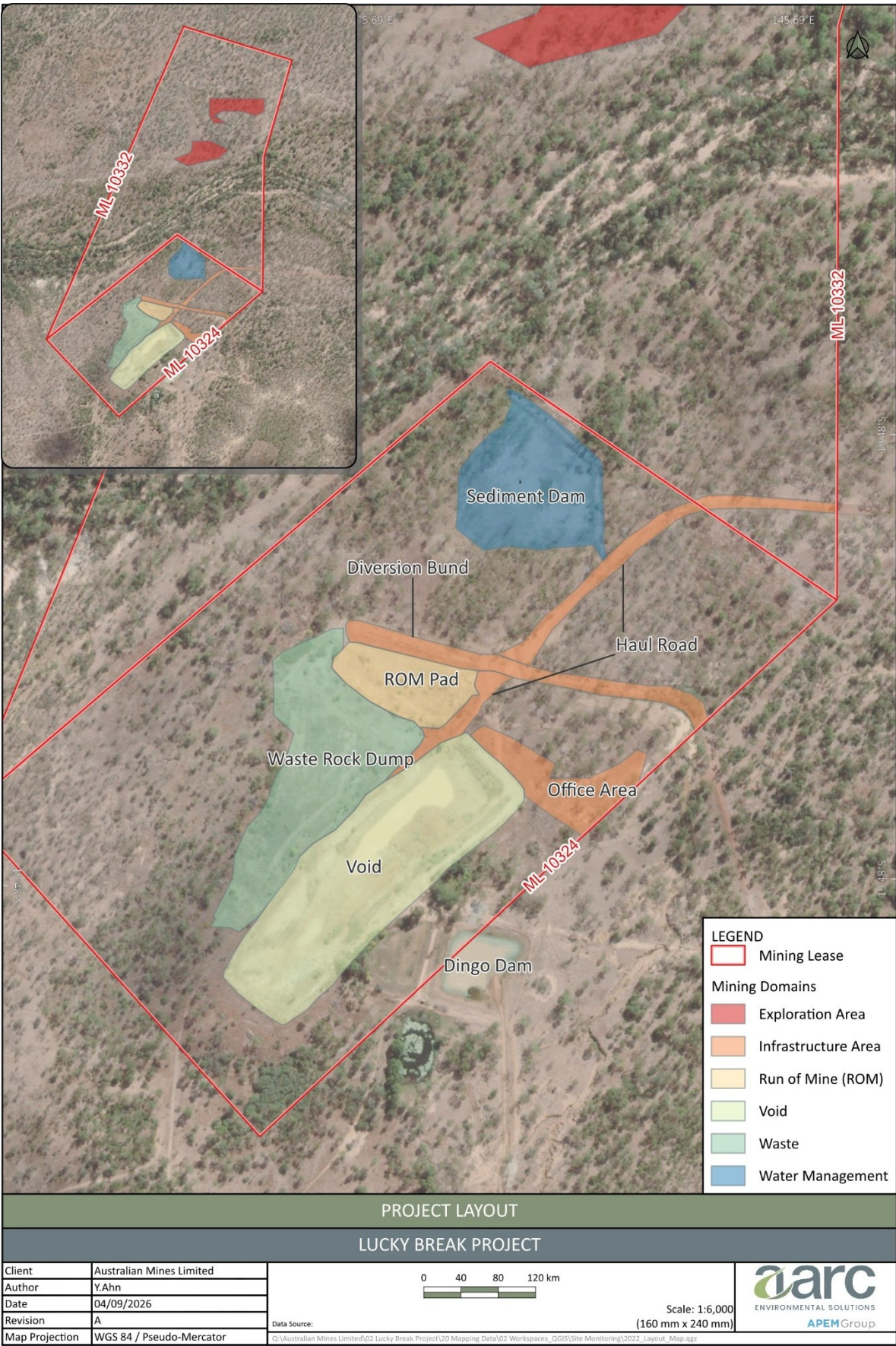
Figure 2: Project layout prior to rehabilitation
