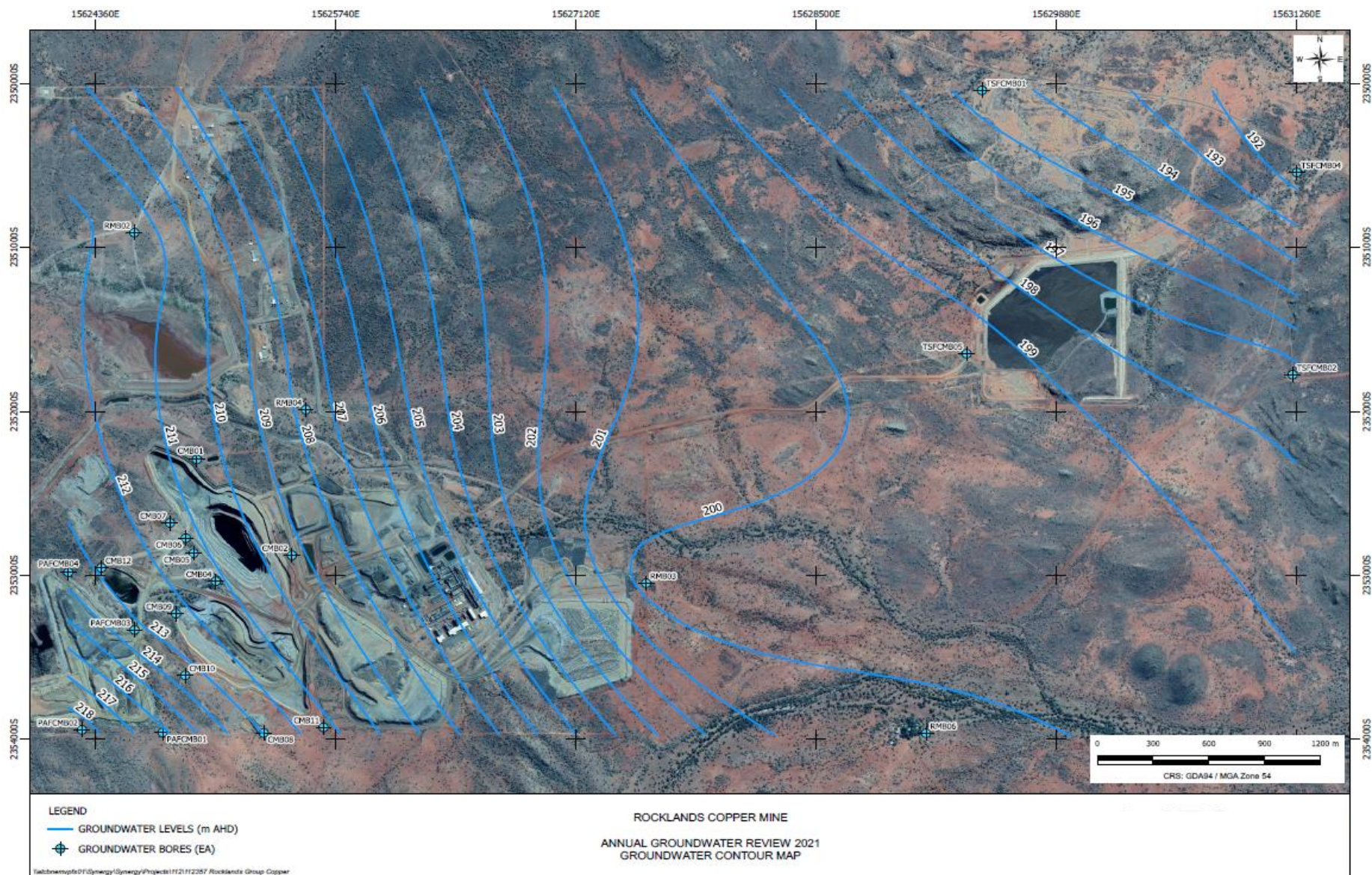
Figure 3.3: Groundwater Contour Map 2021 (Figure 005, ATCW 2022)
