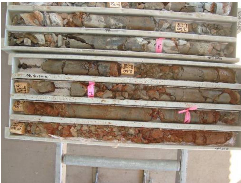
Plate 1: Borehole PS S04 –0.0 to 2.80 m depth.
