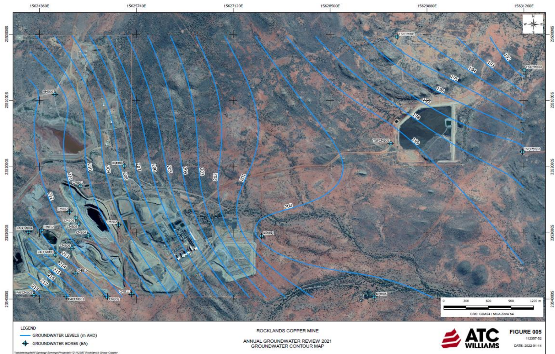
Figure 2.12: Groundwater Level Contours and Flow Direction (ATCW2022b).
