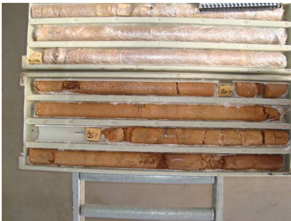
Plate 1: Borehole TSF02 –0.0 to 3.10 m depth.
