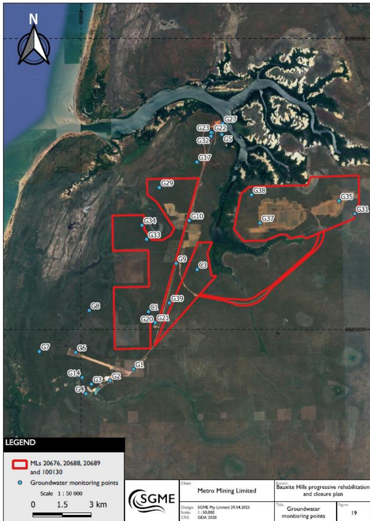
Figure 4. Groundwater monitoring locations
