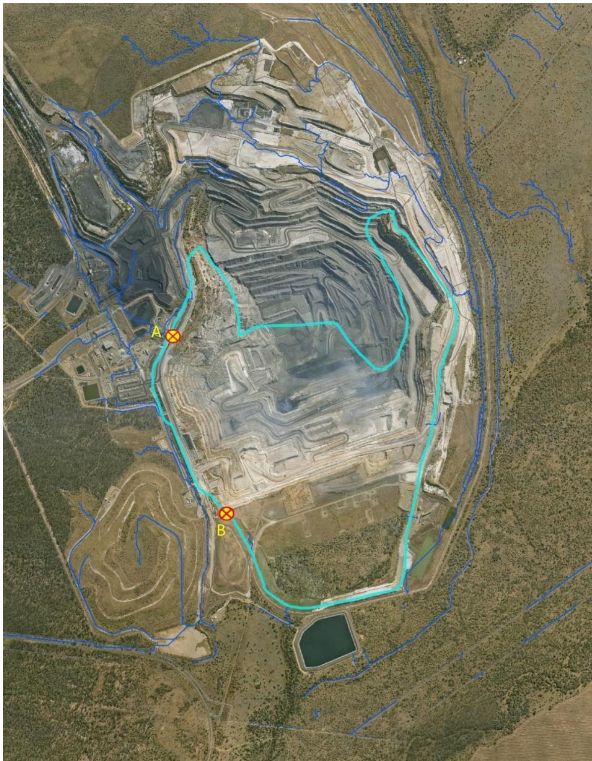
Figure 3 – Highwall segment permitted to achieve FoS \geq 1.3
