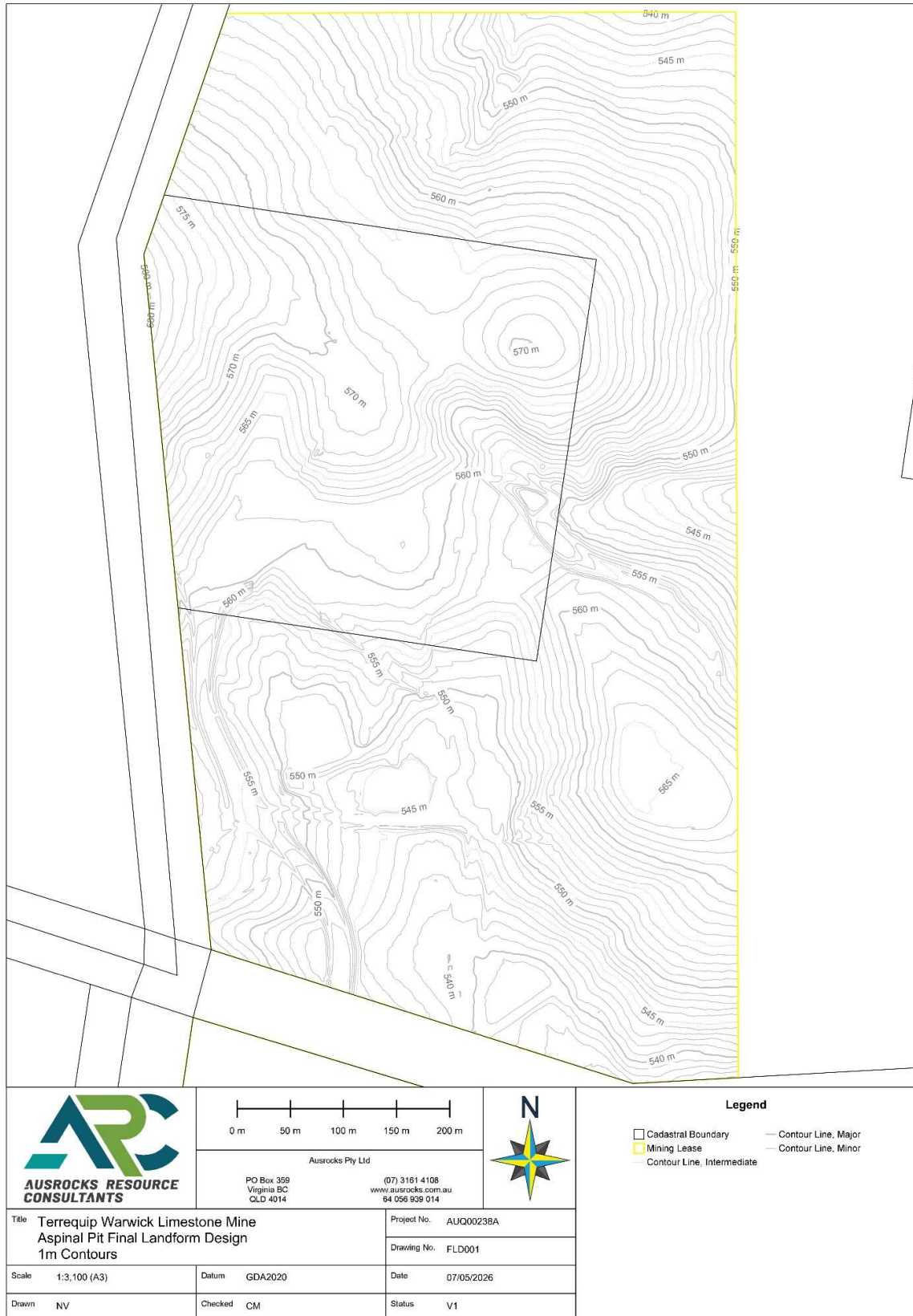
Figure 20: Aspal Pit Final Landform Design (1m contours)
