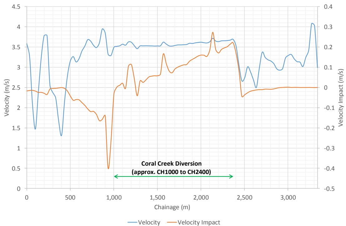
Figure 5.2 Incremental 1:1,000 AEP Flood Velocity Impact – Long Section
