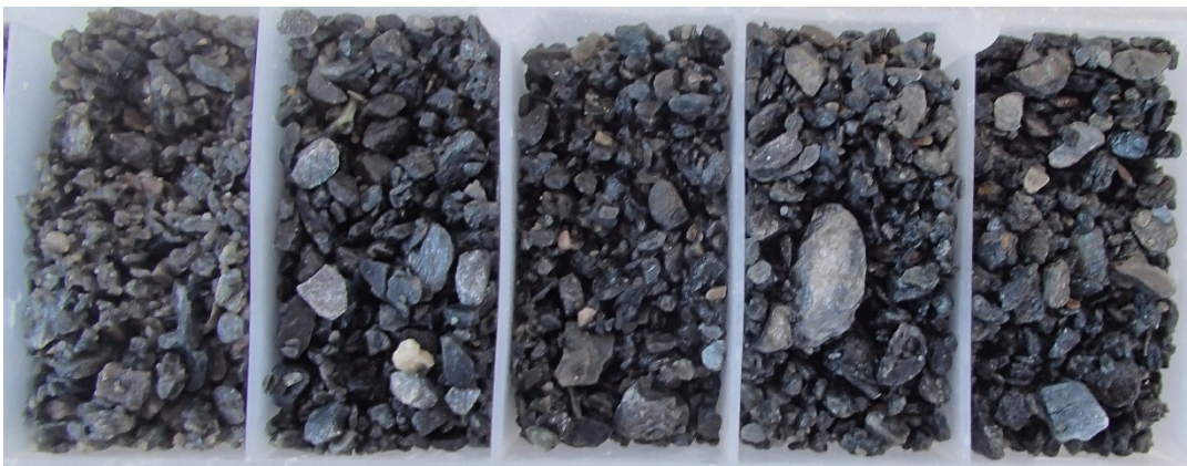
Photograph II-28: BSOC_B5 Drill Cuttings, 30-35m; End of Hole.
