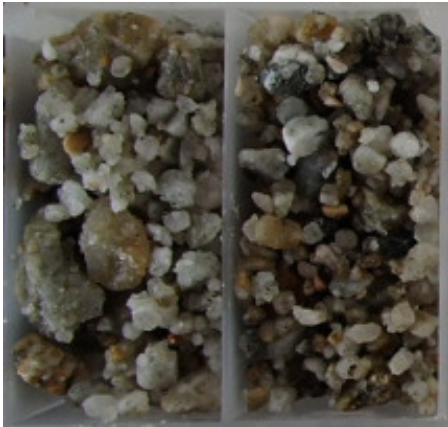
Photograph II-10: BSOC_B2 Drill Cuttings, 24-26m; End of hole.
