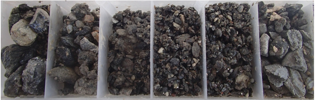
Photograph II-17: BSOC_B4 Drill Cuttings, 0-6m
