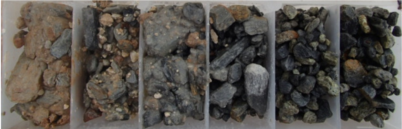
Photograph IV-1: BSOC_B1 Drill Cuttings, 0-6m
