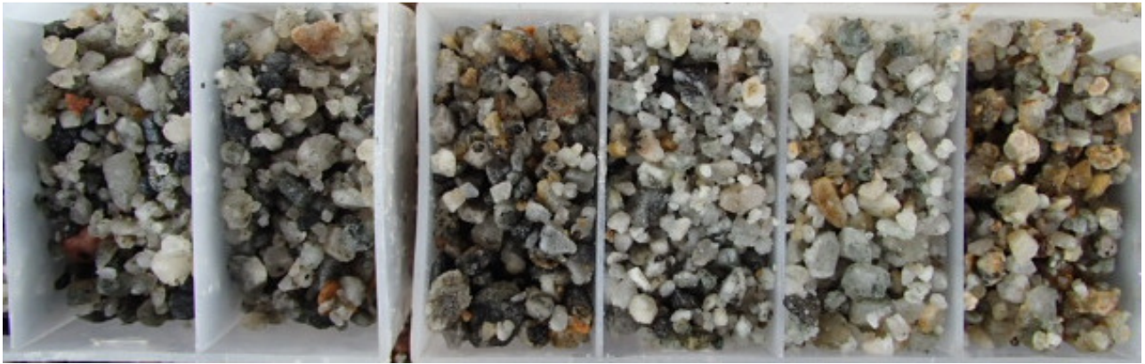
Photograph II-9: BSOC_B2 Drill Cuttings, 18-24m
