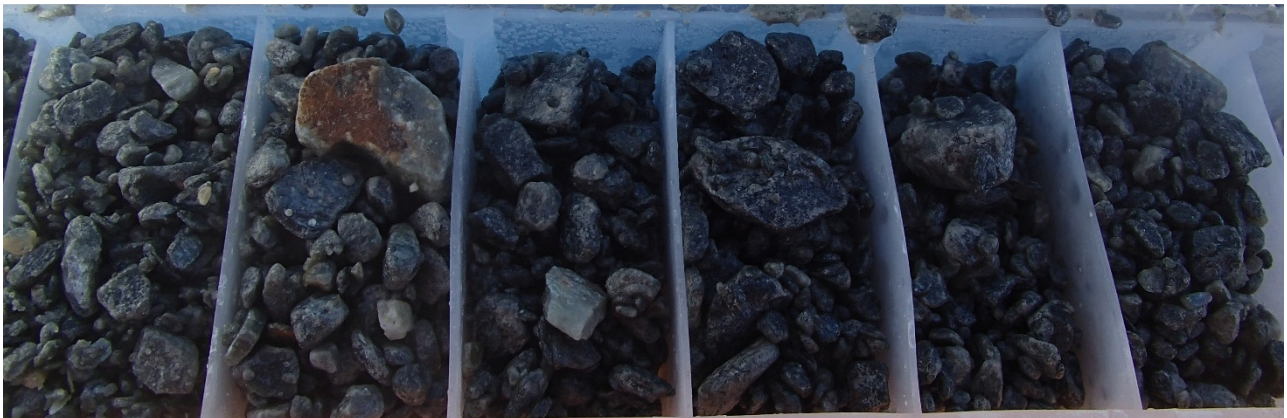
Photograph II-40: BSOC_B6 Drill Cuttings, 66-72m; End of hole.
