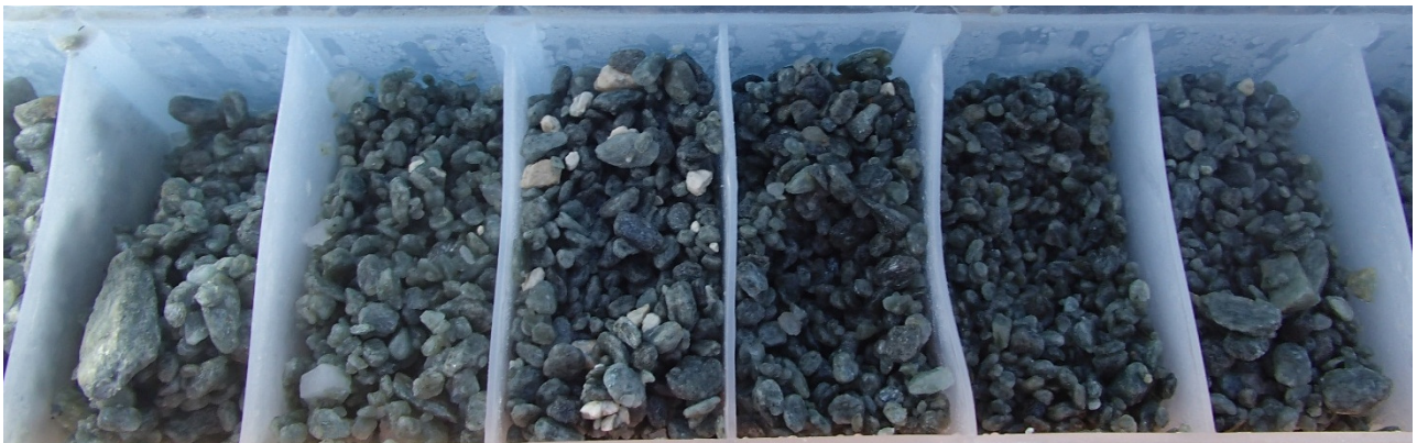
Photograph II-30: BSOC_B6 Drill Cuttings, 6-12m
