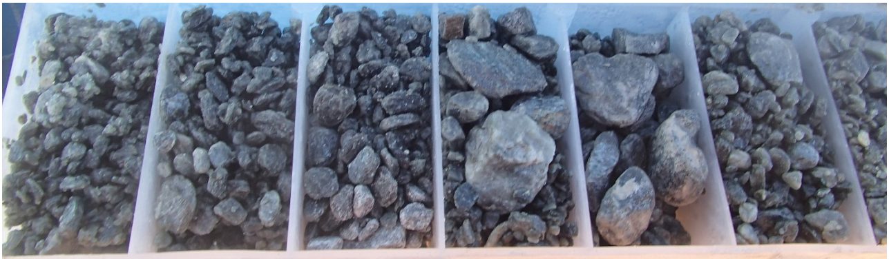
Photograph II-39: BSOC_B6 Drill Cuttings, 60-66m
