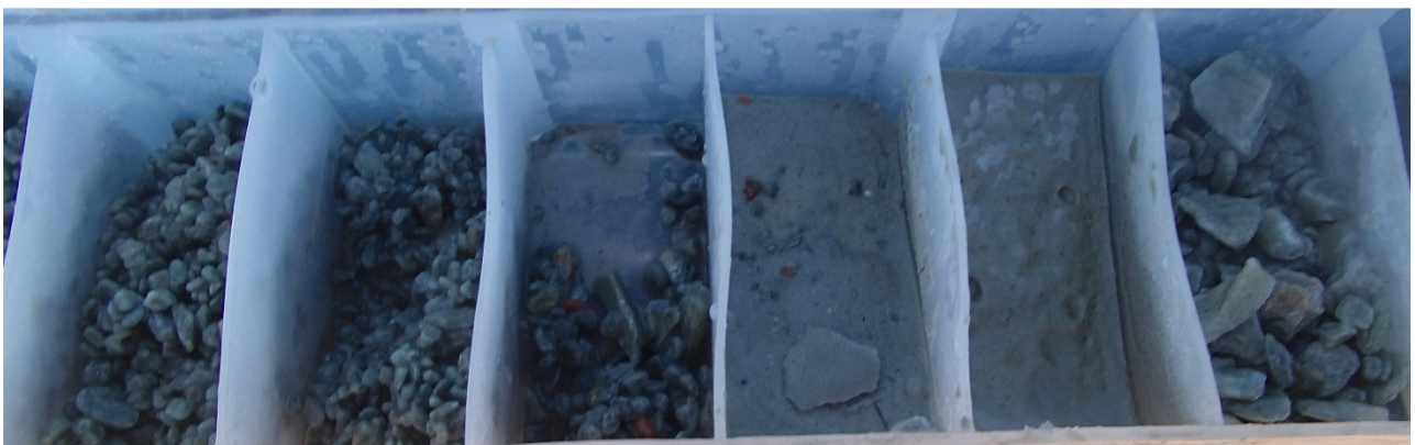
Photograph II-31: BSOC_B6 Drill Cuttings, 12-18m
