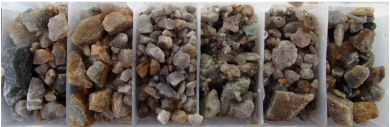
Photograph II-7: BSOC_B2 Drill Cuttings, 6-12m
