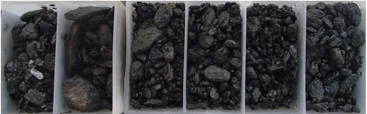
Photograph II-20: BSOC_B4 Drill Cuttings, 18-24m
