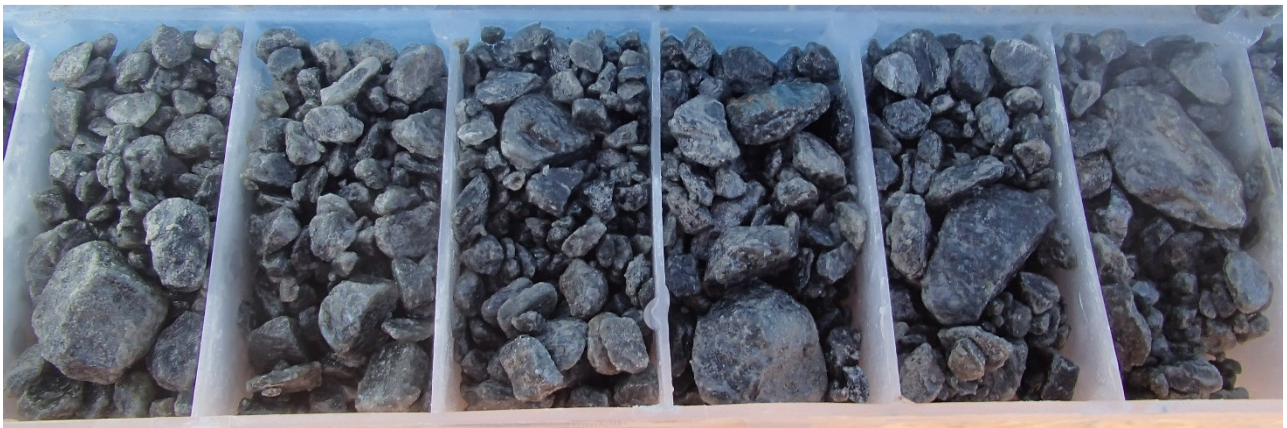
Photograph II-36: BSOC_B6 Drill Cuttings, 42-48m
