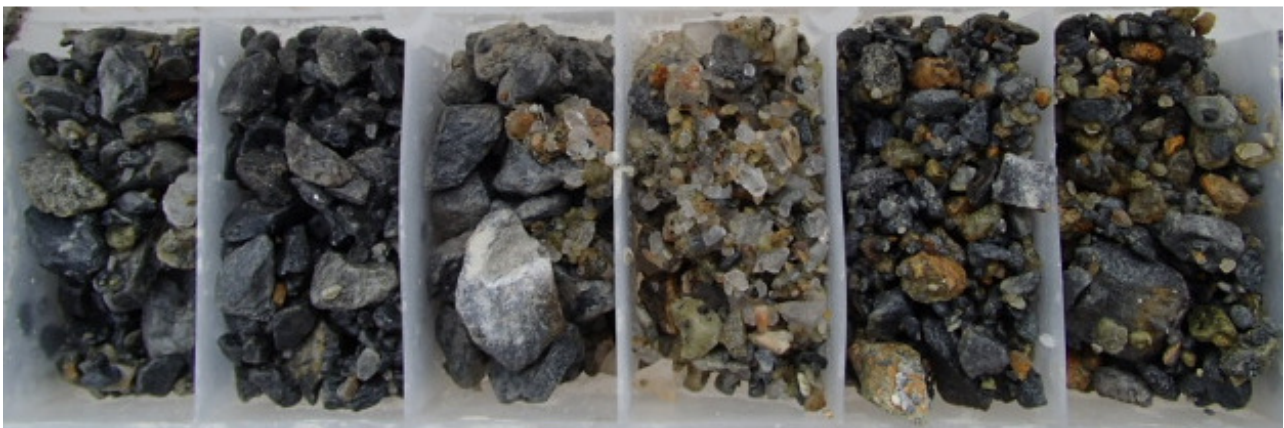
Photograph IV-2: BSOC_B1 Drill Cuttings, 6-12m
