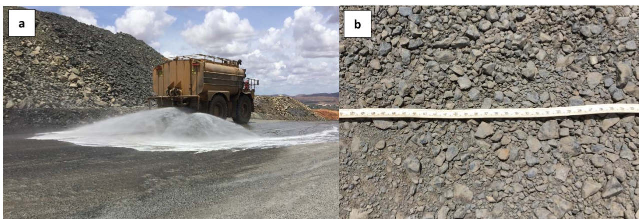
Figure 5-24: Infiltration observations on highly trafficked / compacted area. a) water infiltration test, b) compacted waste rock surface (December, 2015)
