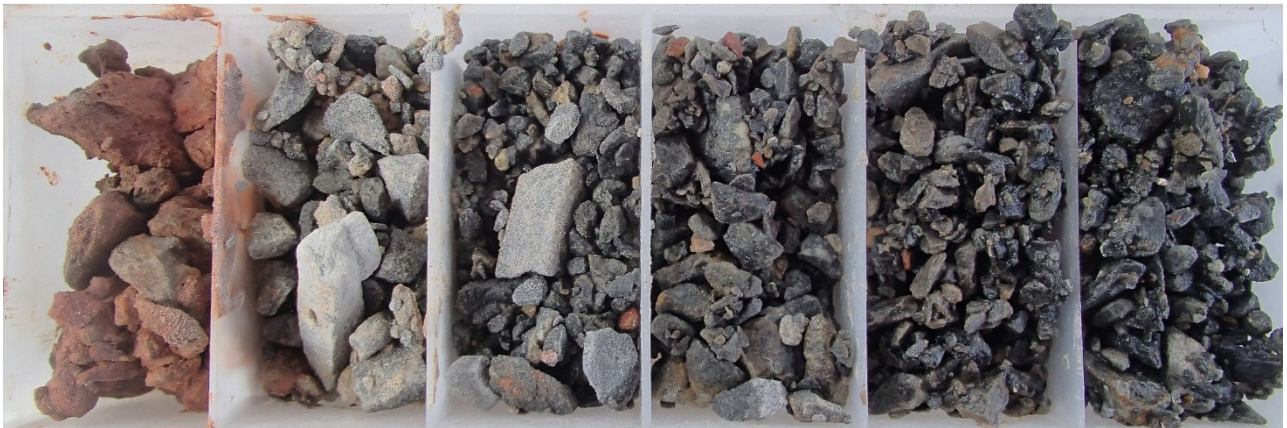
Photograph II-11: BSOC_B3 Drill Cuttings, 0-6m
