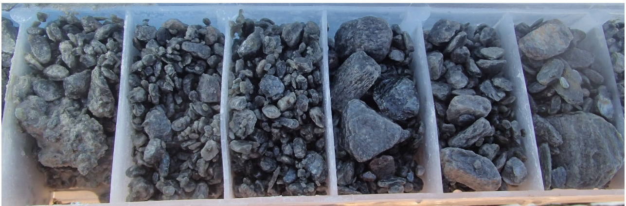
Photograph II-37: BSOC_B6 Drill Cuttings, 48-54m
