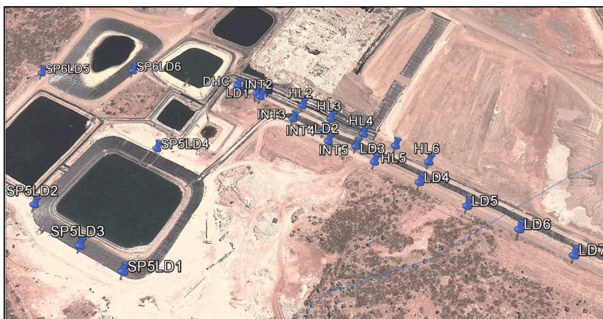
Figure 20 Location of Leak Detection (LD) Bores in the area of the Heap Leach Facility and associated dams
