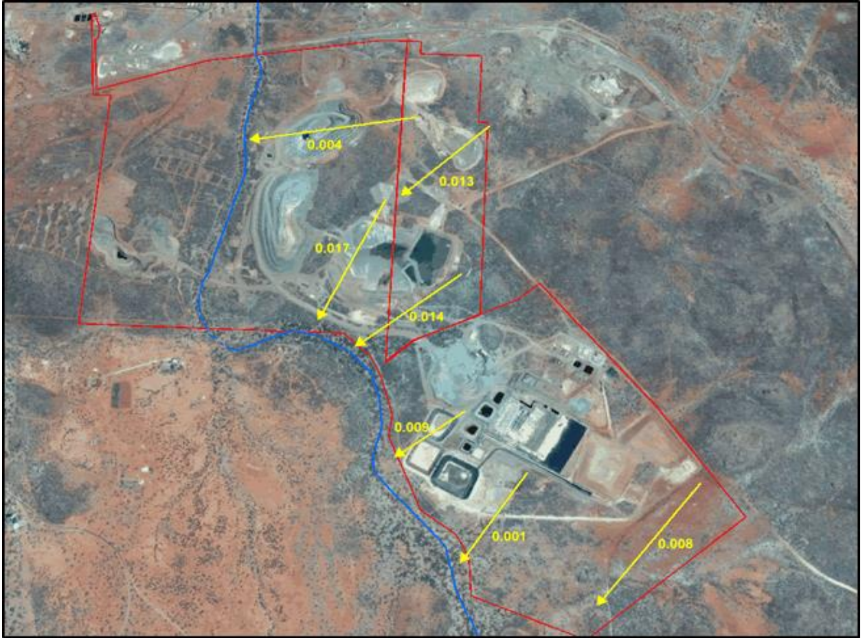
Figure 4: Generalised direction of groundwater flow and calculated hydraulic gradients (i.e. 0.008). Note: The yellow arrows denote the generalised direction of groundwater flow (calculated using groundwater levels from two distinct bores) and not actual groundwater flow-lines.
