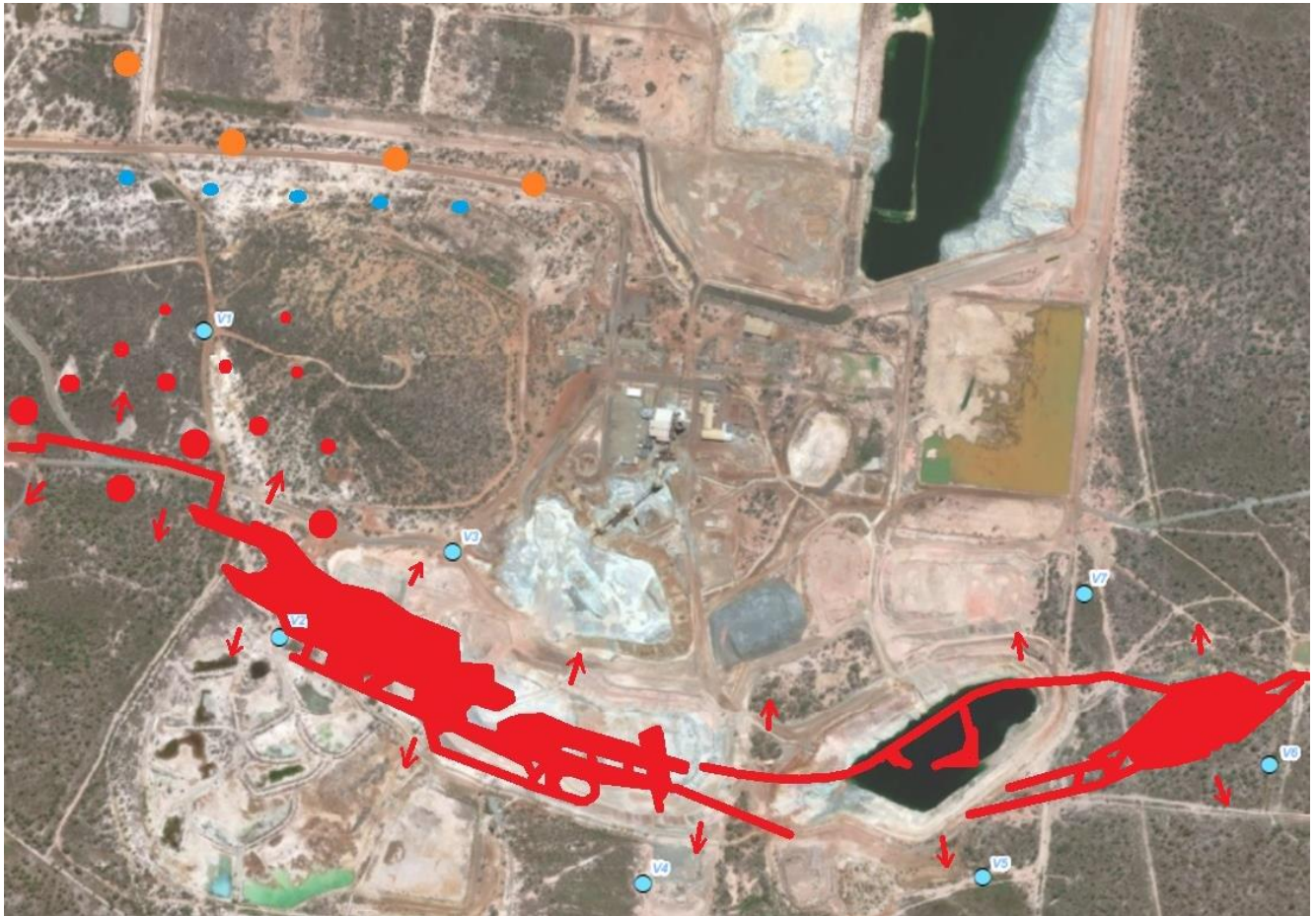
Figure 78 Schematic depiction of the increase in groundwater levels induced by tailings and process water deposition to the Central pit and former underground prior to 2008 (Red arrow- direction of groundwater flow; Orange-Tailings seepage; Red- migration of underground backfill seepage; Blue – natural groundwater. Size of circle anticipated concentrations)
