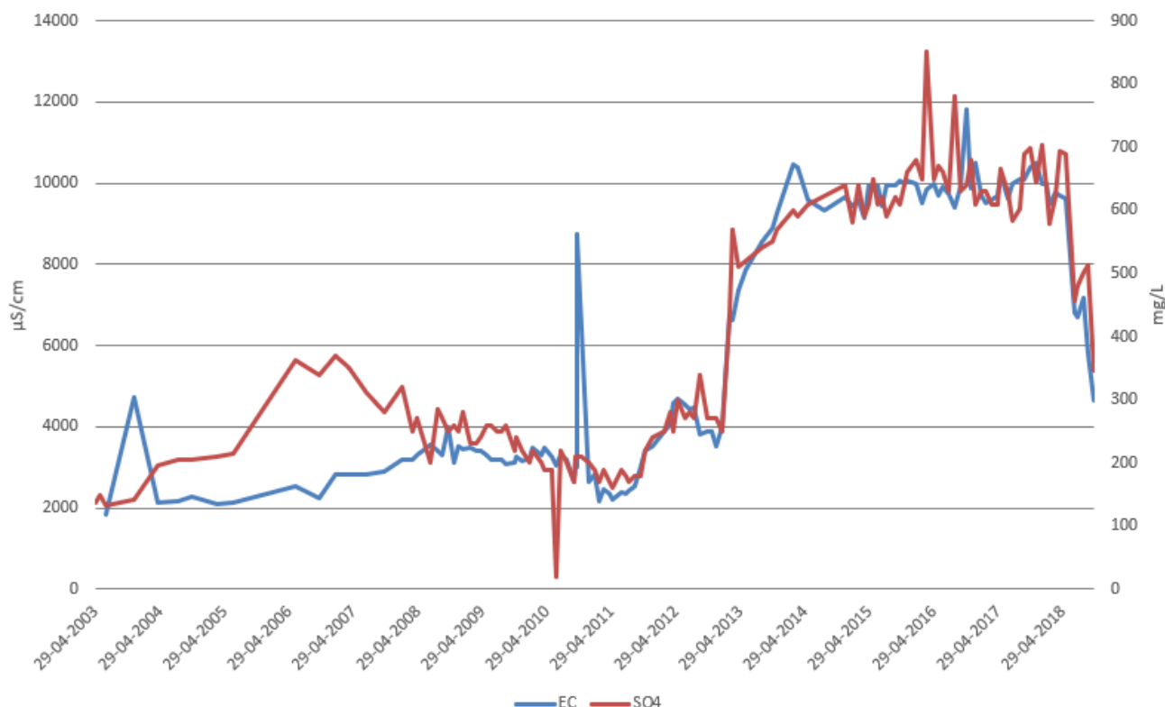
Figure 77 EC (µS/cm) and sulfate (mg/L) development at V1 between installation in 2003 and October 2018
