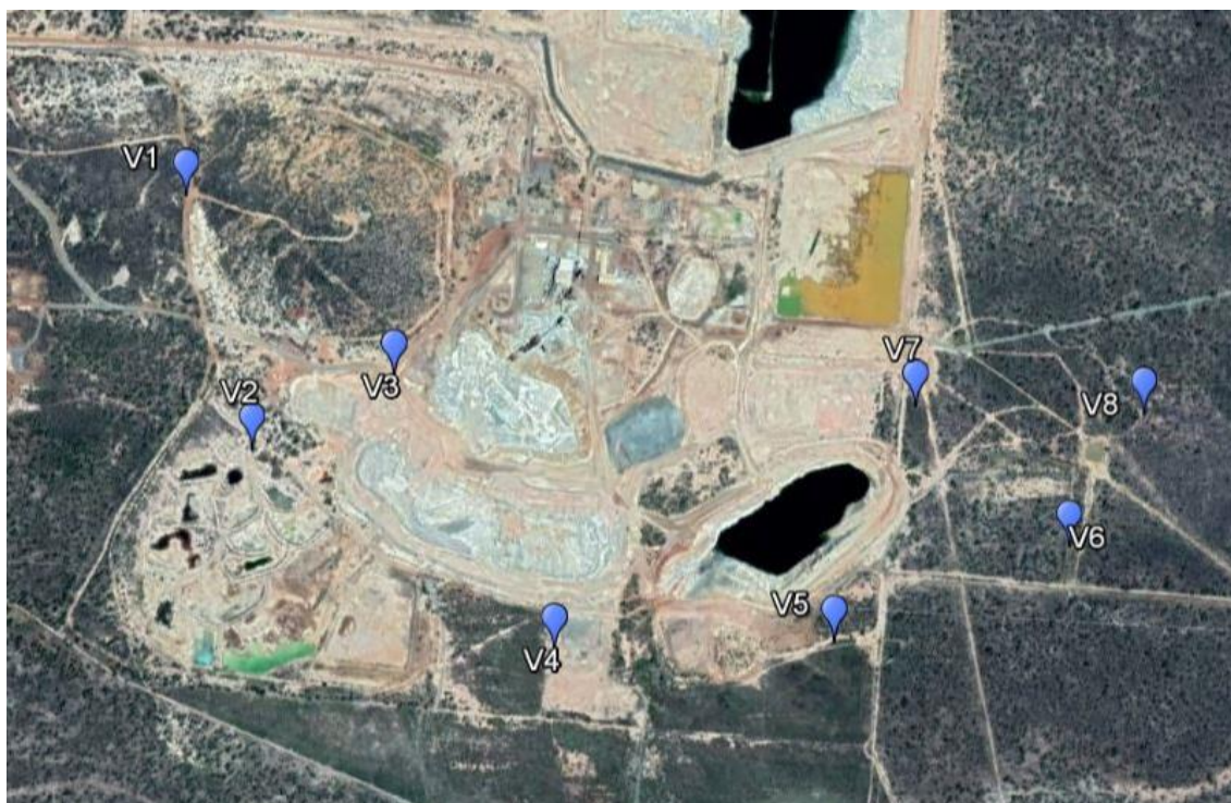
Figure 15 Location of the 2003 V series bores to monitor the impact of underground tailings deposition
