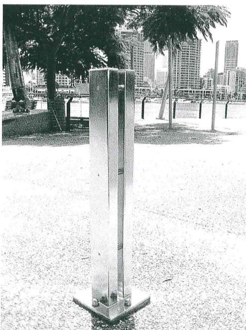
Electropolished stainless steel grade 316 in perfect condition after 7 years of exposure in a marine environment.
