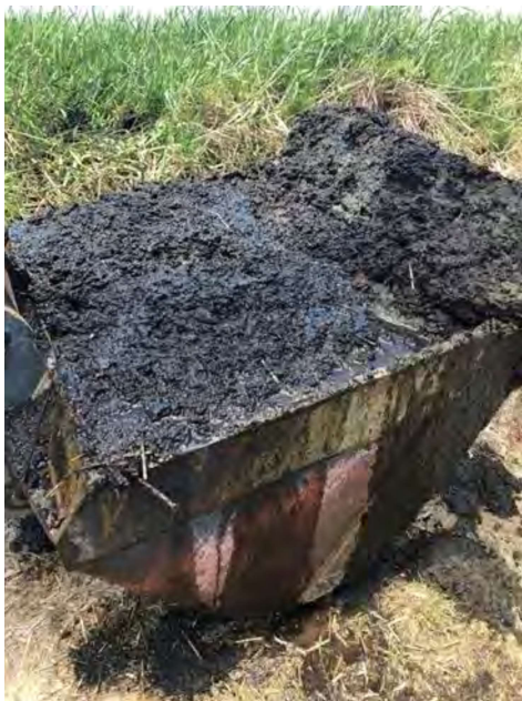
Photograph 2.1: Sludge sample collected using long reach excavator
