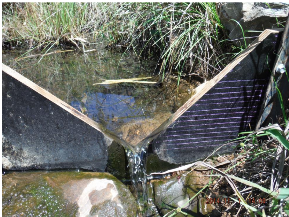
Photograph of v-notch weir at 1 st November 2014
