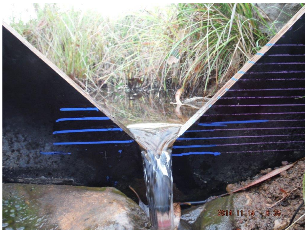
Photograph of v-notch weir at 14 th November 2014
