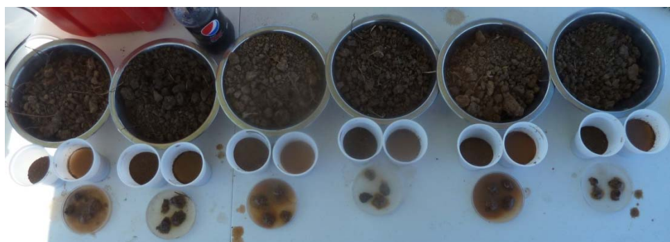
Figure 7 Slaking and dispersion in dam wall samples 15-17
