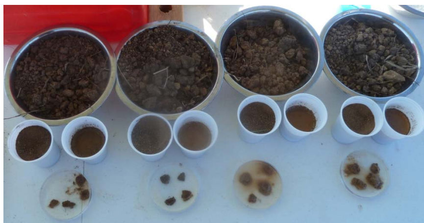
Figure 6 Slaking and dispersion in dam wall samples 13 and 14
